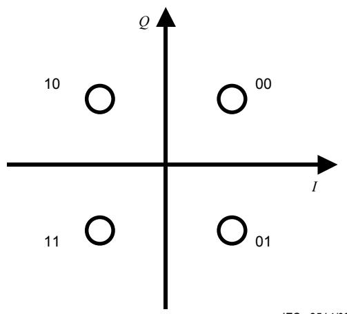
**Figure 20 – QPSK mapping**
