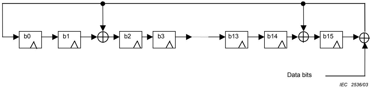
**Figure B.3 – Linear feedback shift register circuit****B.1.2.1.12 Padding\_bits**
