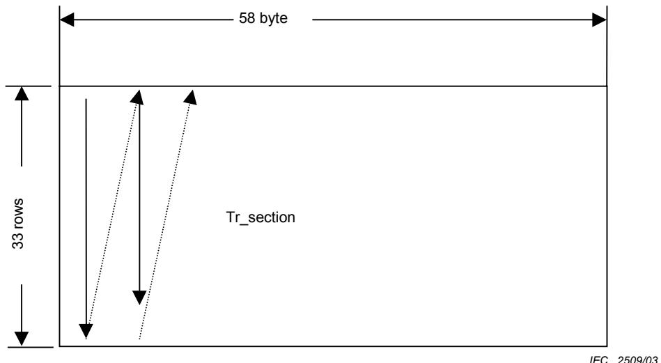
**Figure 15 – The order bytes in Tr\_section**
