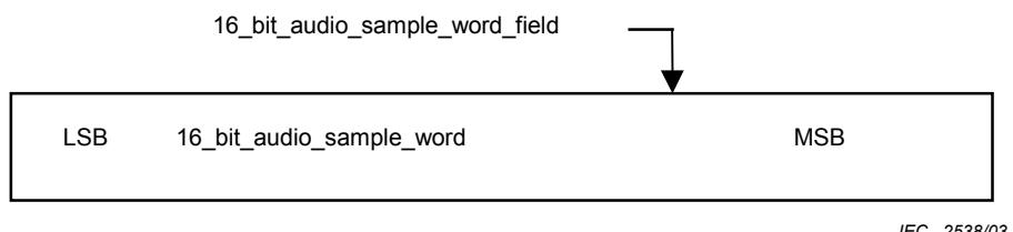
**Figure B.5 – Sub-frame structure of half-band mode**
