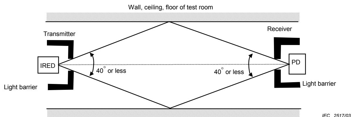
**Figure 23 – Location for measurements**
