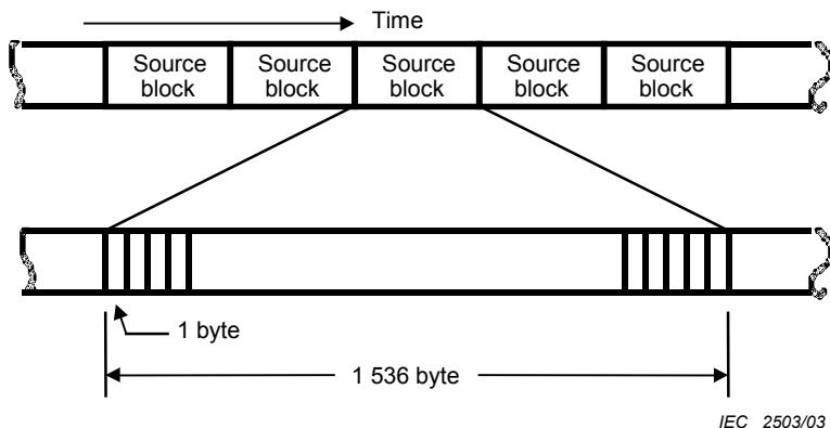
**Figure 9 – Source\_block stream**
