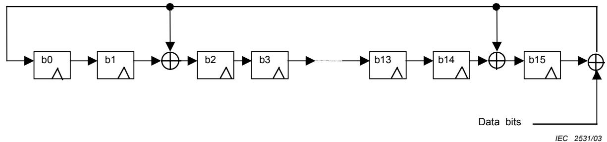
**Figure A.3 – Linear feedback shift register circuit**
