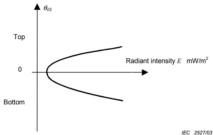
**Figure 31b – Vertical directivity****Figure 31 – Directivity characteristics of the receiver**
