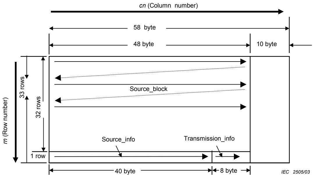
**Figure 11 – Block alignment**
