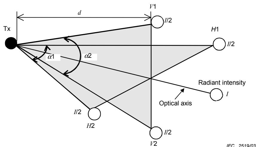
**Figure 25 – Angle of half optical radiant intensity**
