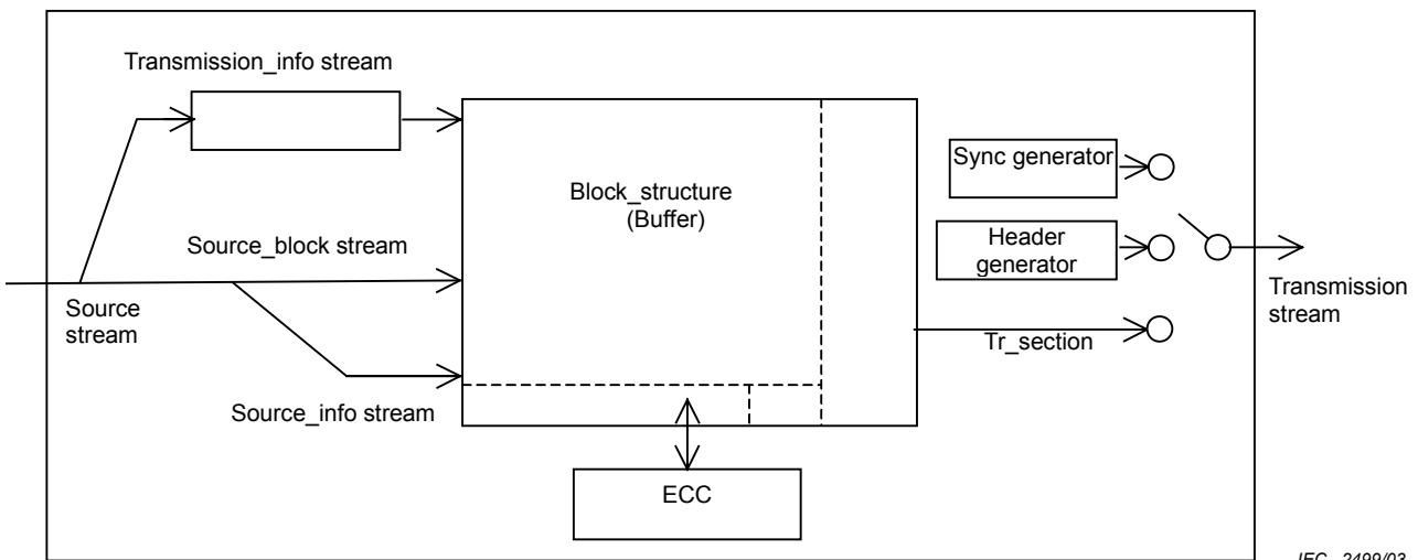
**Figure 5 – Channel-coding block**
