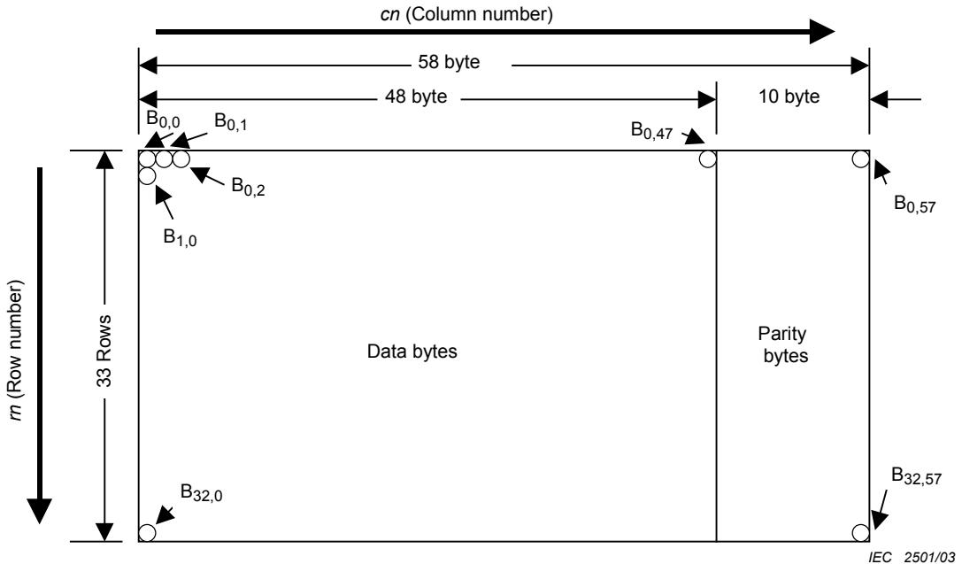
**Figure 7 – Block structure**
