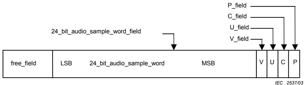
**Figure B.4 – Sub-frame structure of full-band mode****B.2 Half-band mode****B.2.1.1 Syntax of half-band mode**
