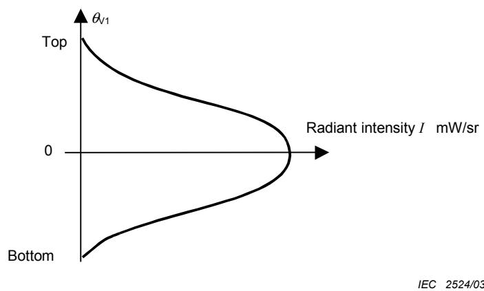
**Figure 29b – Vertical directivity****Figure 29 – Directivity characteristics of the transmitter**
