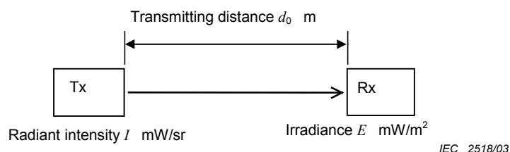
**Figure 24 – Transmitting distance**
