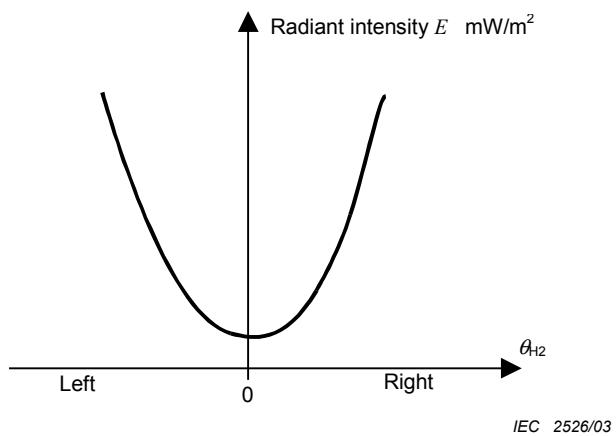
**Figure 31a – Horizontal directivity**
