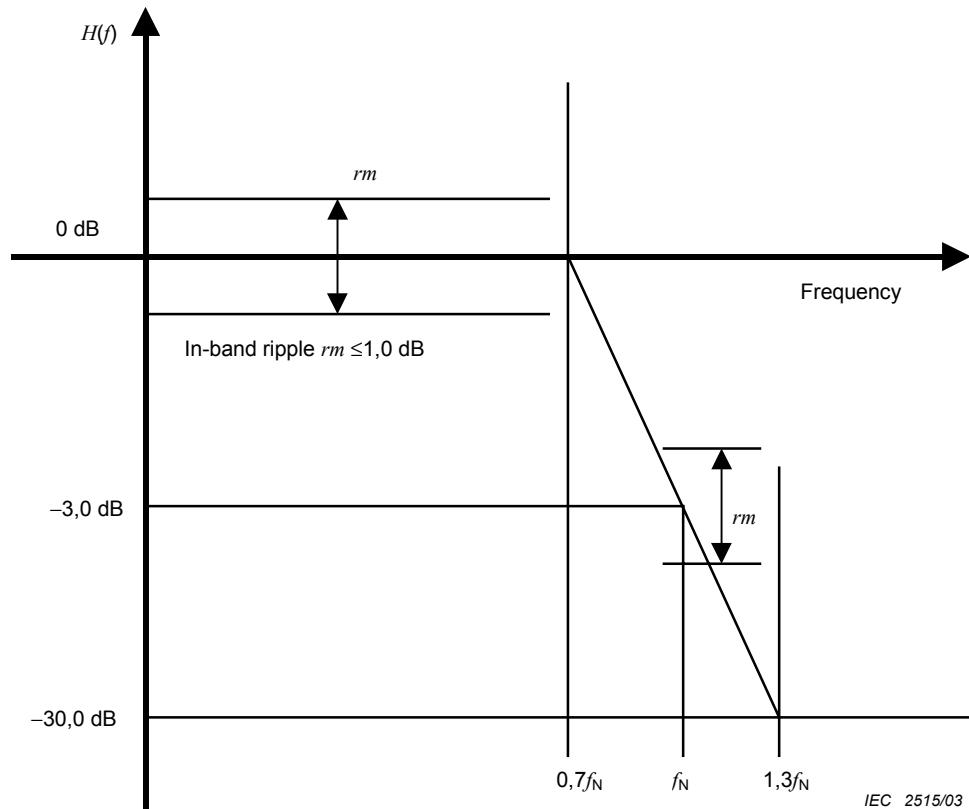
Figure 21 – Baseband filter characteristics
