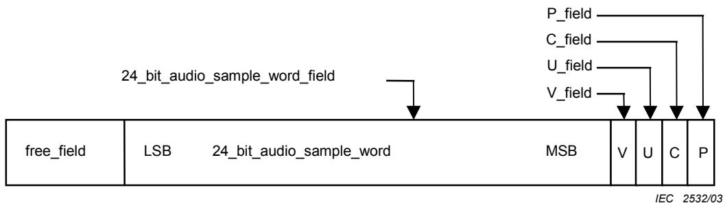
**Figure A.4 – Sub-frame structure of full-band mode**
