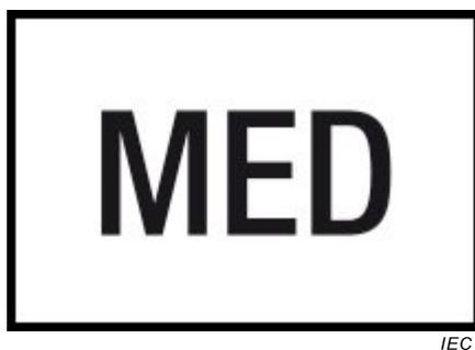
Figure A.1 – Pictogram for marking a MED-IMD
