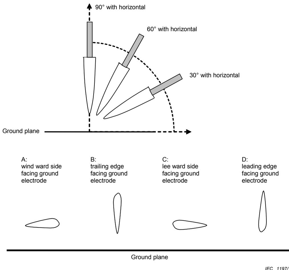
**Figure D.2 – Possible orientations for the initial leader attachment test setup A**
