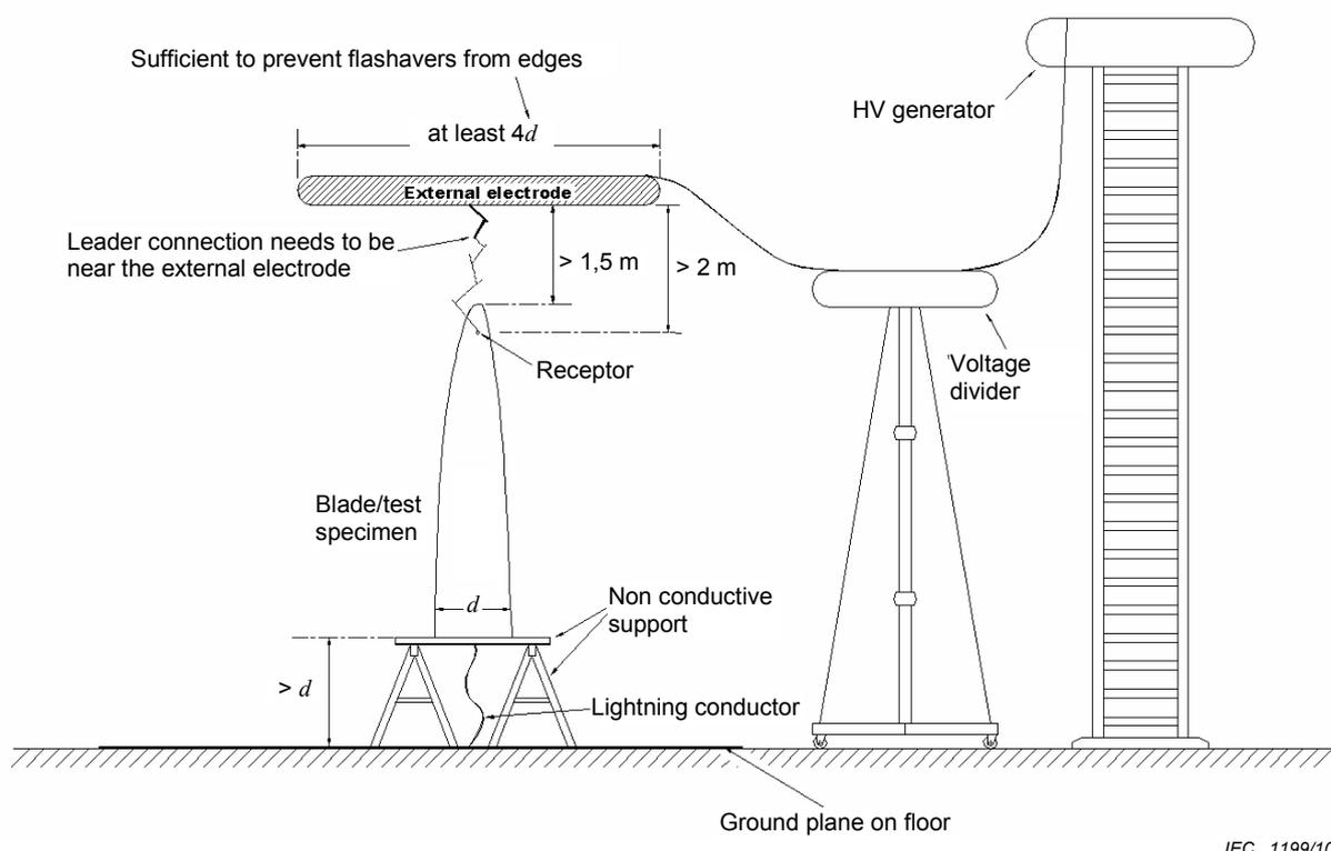
**Figure D.4 – Initial leader attachment test setup B**
