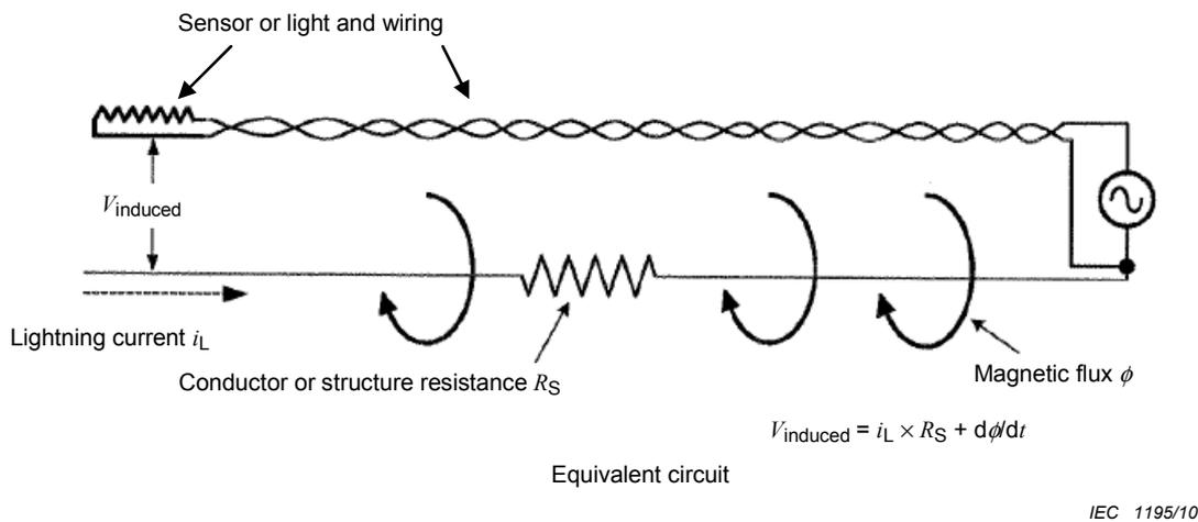
**Figure C.3 – Lightning induced voltages between lightning conductor or structure and sensor wiring**
