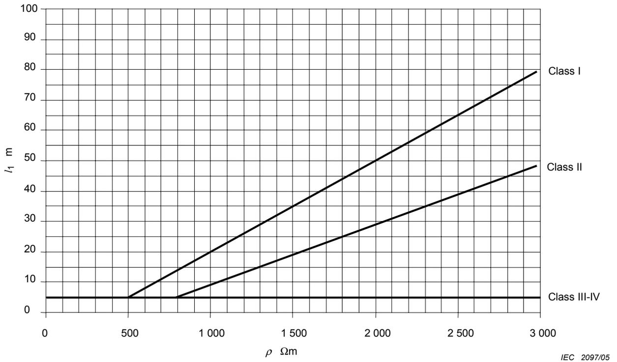
**Figure I.1 – Minimum length ( $l_1$ ) of each earth electrode according to the class of LPS (Figure 2 in IEC 62305-3)**
