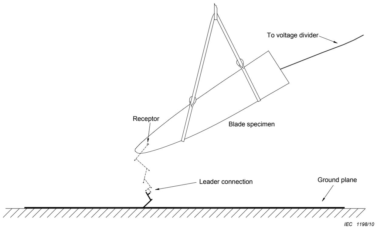
**Figure D.3 – Leader connection point must be away from test specimen**
