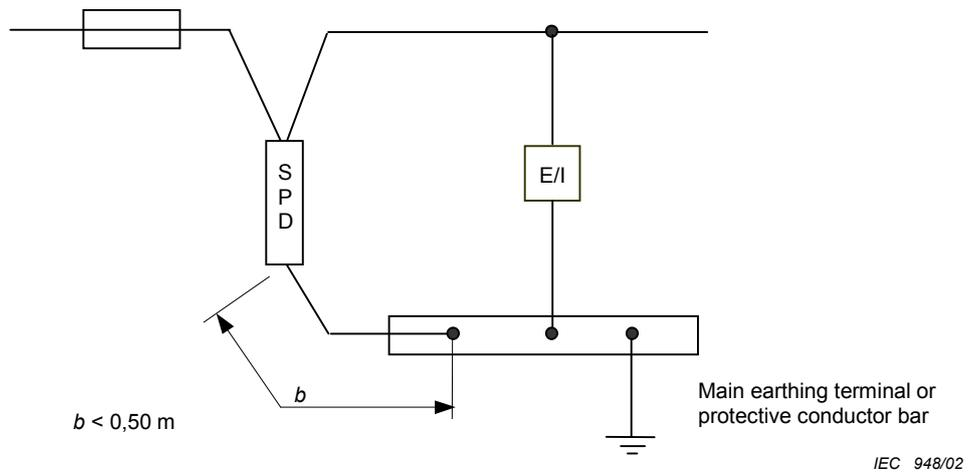
**Figure F.1 – Point-to-point installation scheme**
