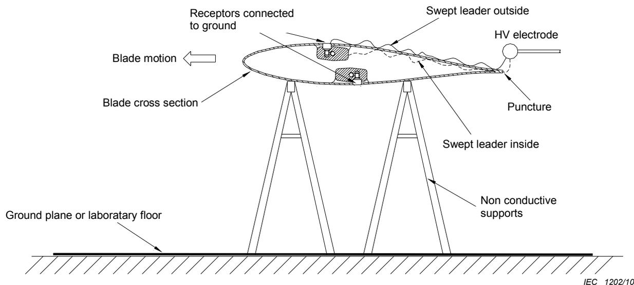
Figure D.7 – Swept channel test arrangement
