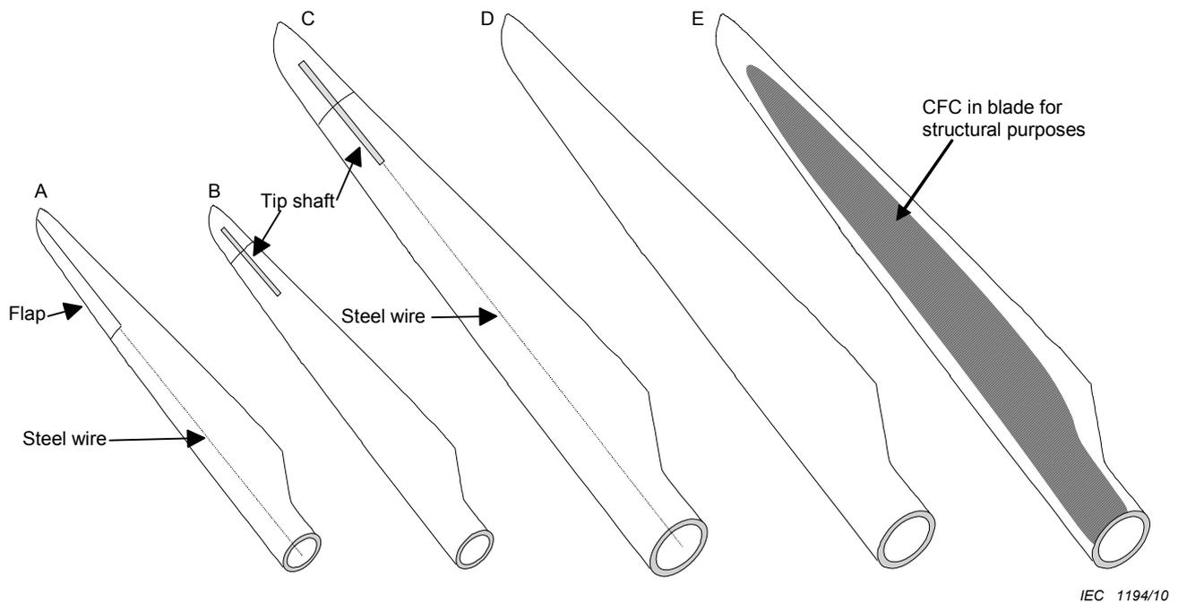
**Figure C.1 – Types of wind turbine blades**
