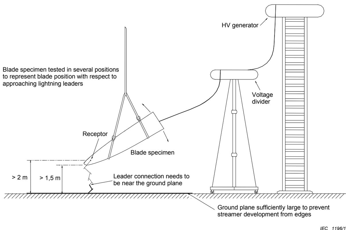
**Figure D.1 – Initial leader attachment test setup A (specimen should be tested in several positions representing different directions of the approaching leader)**
