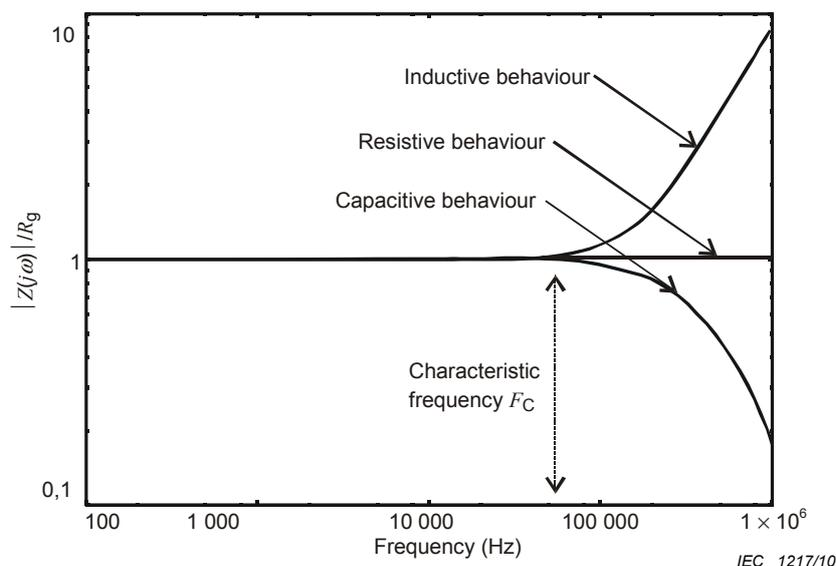
**Figure I.2 – Frequency dependence on the impedance to earth (adapted from Cigré WG C.4.4.02 July 2005 [49])**
