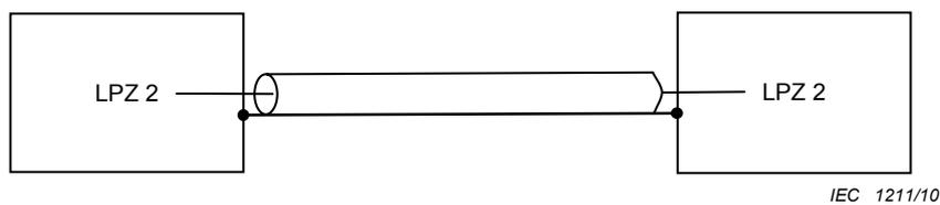
**Figure E.4 – Two cabinets both defined as LPZ 2 connected via the shield of a shielded cable**
