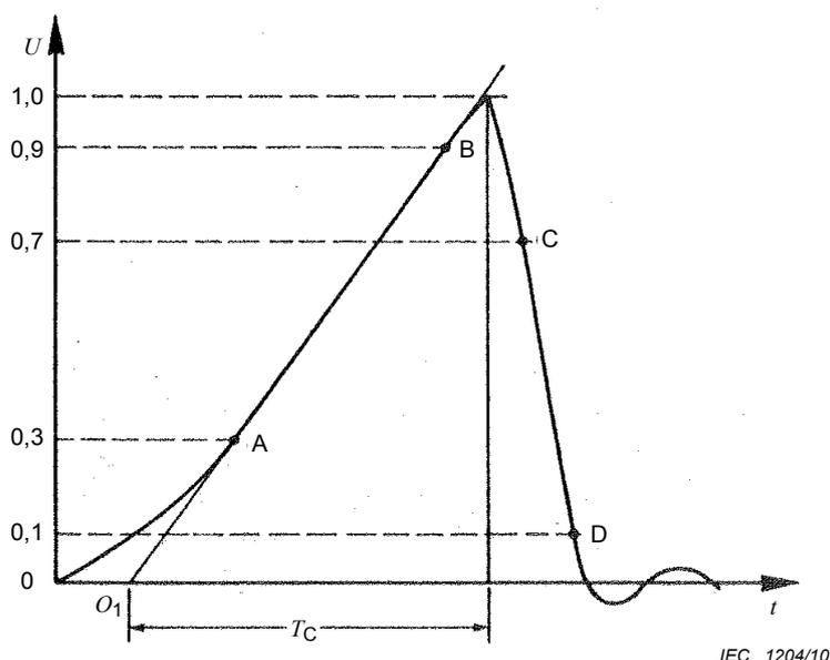
**Figure D.9 – Lightning impulse voltage waveform showing flashover on the wave front (Figure 7 in IEC 60060-1)**
