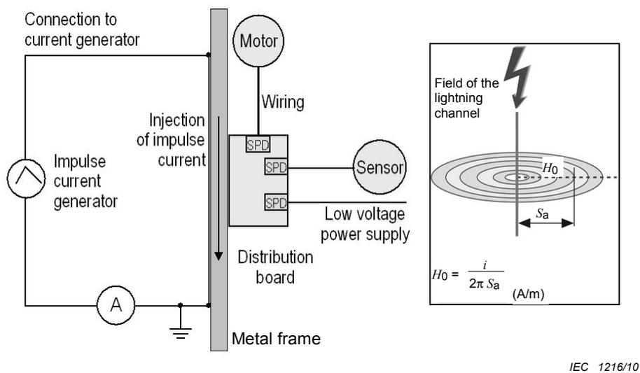
Figure H.2 – Example circuit of an induction test due to lightning currents
