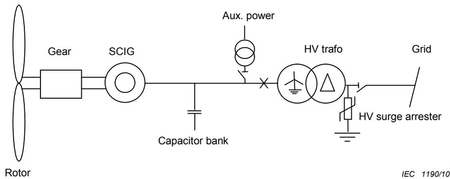
Figure 4a – Squirrel cage induction generator (SCIG)
