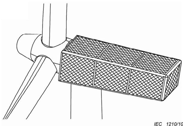
**Figure E.3 – Mesh with small mesh dimension for nacelle with GFRP cover**
