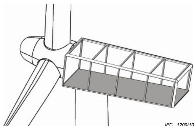
**Figure E.2 – Mesh with large mesh dimension for nacelle with GFRP cover**
