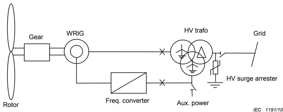
Figure 4b – Wound rotor induction generator (WRIG)
