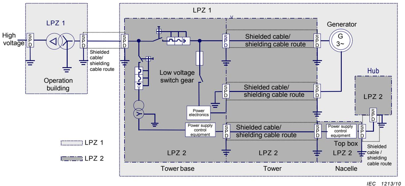
Figure E.6 – Example of how to document LPMS division of electrical system into protection zones with indication of where circuits cross LPZ boundaries and showing the long cables running between tower base and nacelle
