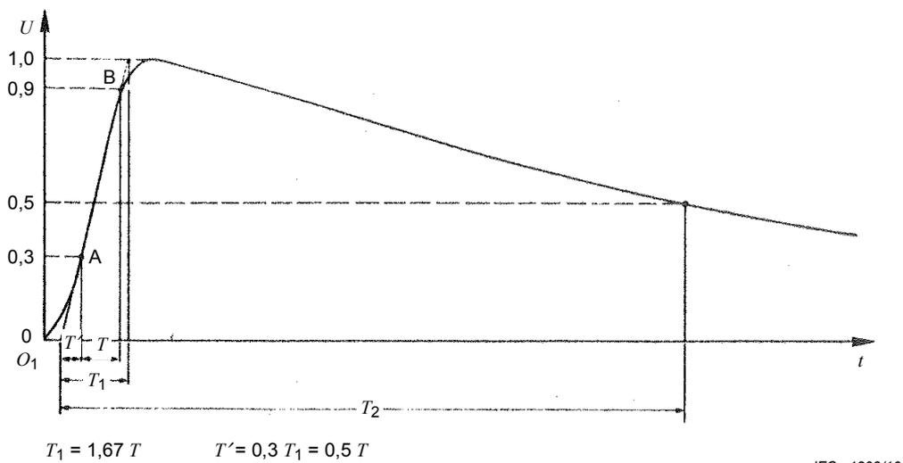
Figure D.8 – Lightning impulse voltage waveform (Figure 6 in IEC 60060-1)
