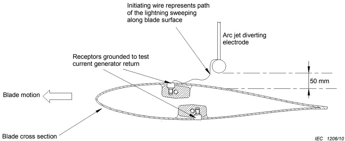
**Figure D.11 – High-current test arrangement for non-conductive surfaces**
