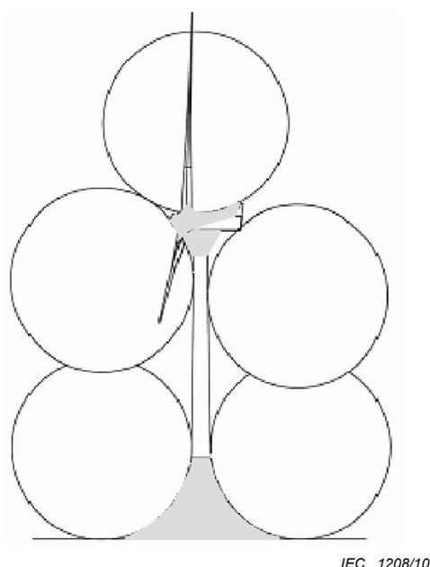
**Figure E.1 – Rolling sphere model**
