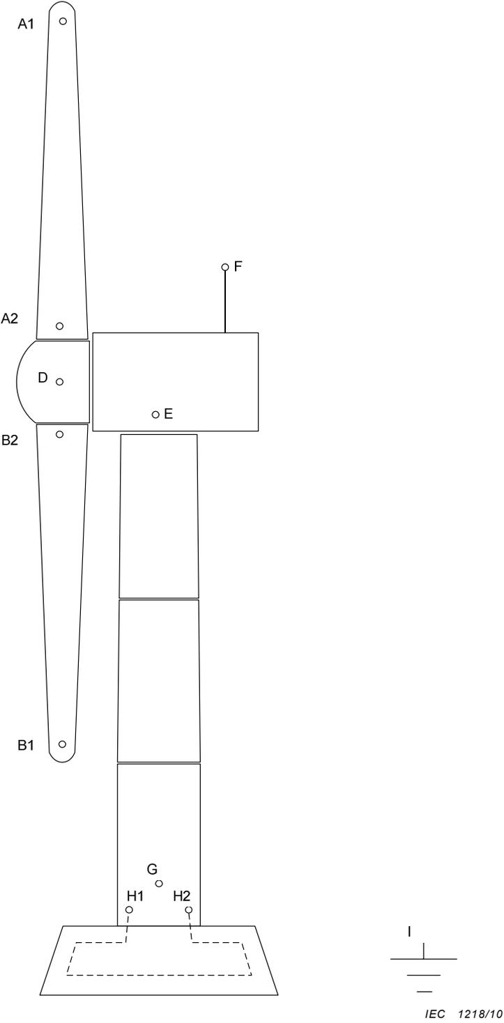
Figure J.1 – Example of measuring points
