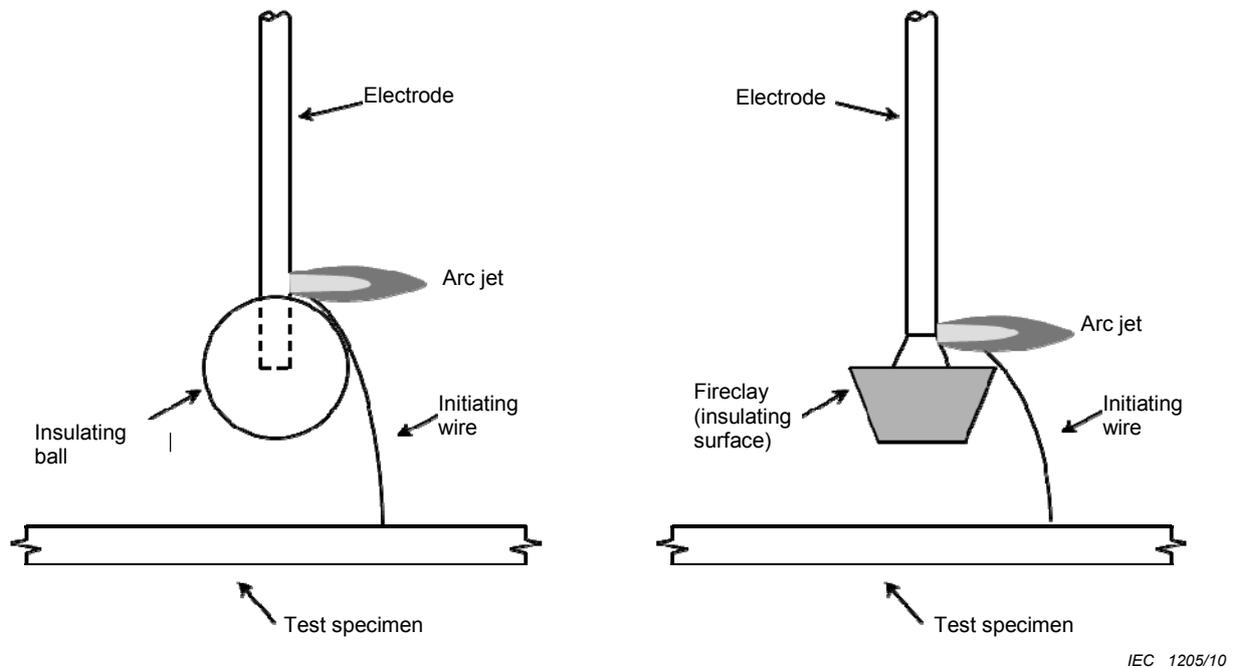
Figure D.10 – Typical jet diverting test electrodes
