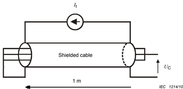
**Figure G.3 – Measuring of transfer impedance**
