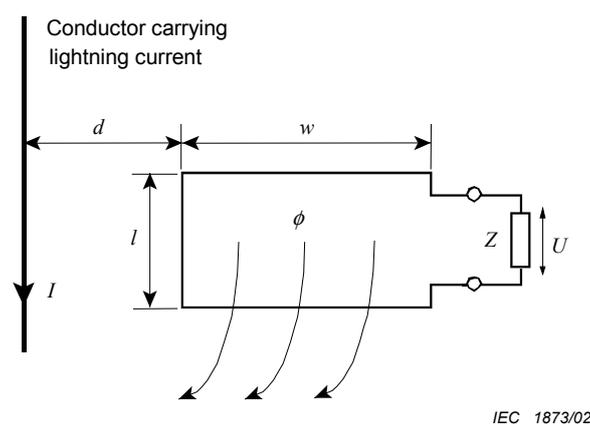
**Figure G.2 – Magnetic coupling mechanism**
