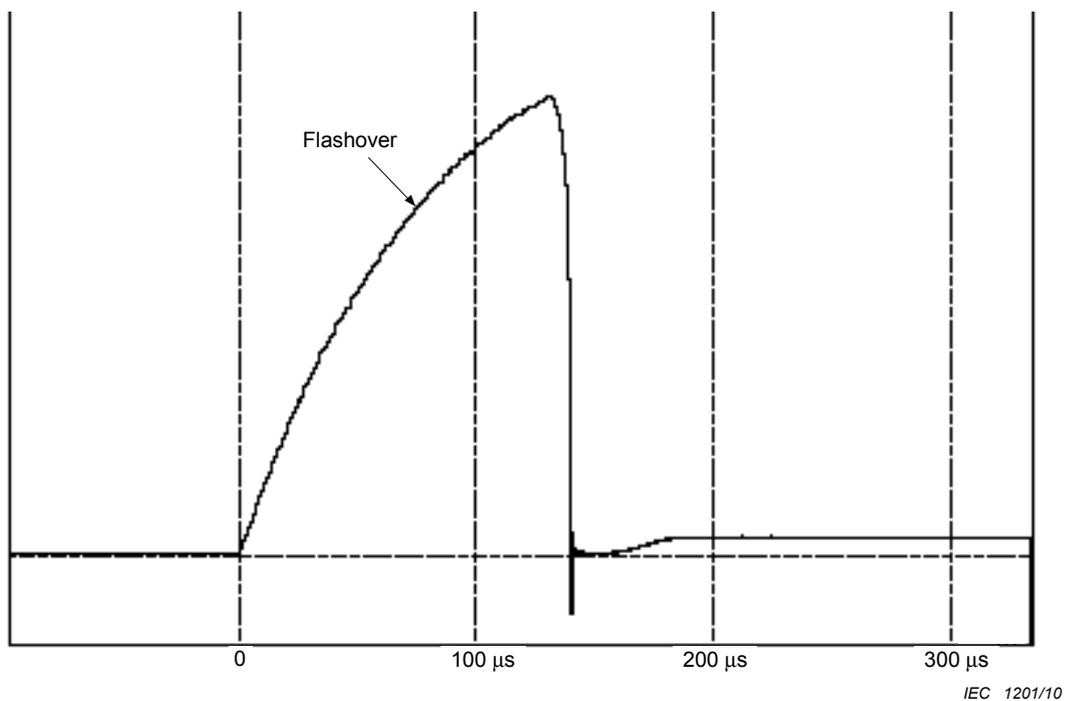
**Figure D.6 – Typical switching impulse voltage rise to flashover (100 μs per division)**
