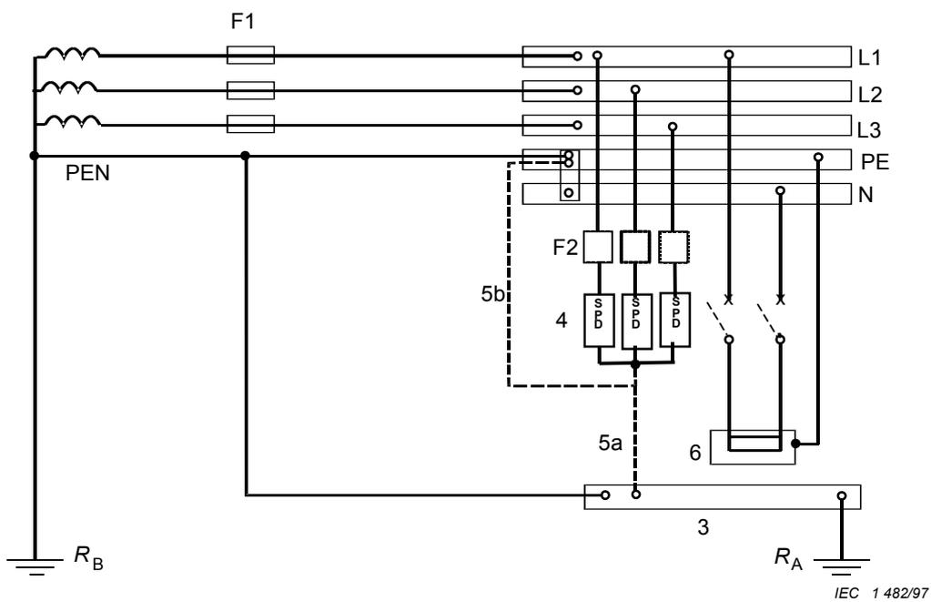
**Figure F.2 – Earthing connection installation scheme**
