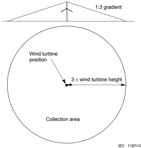
**Figure 1 – Collection area of the wind turbine**
