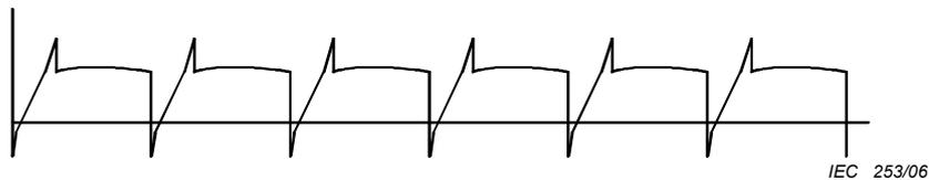
Figure 6e – Self communication: line-to-earth voltage
