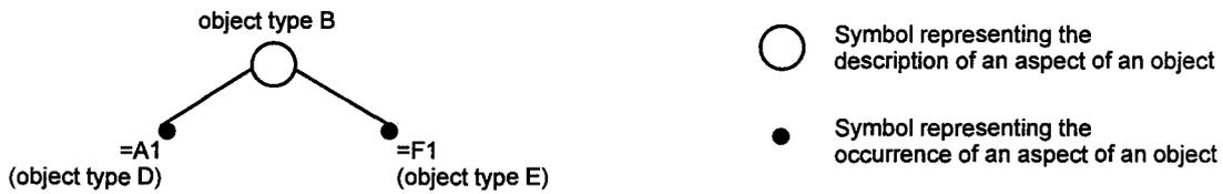
Figure 15 - Function-oriented structure of object type B
