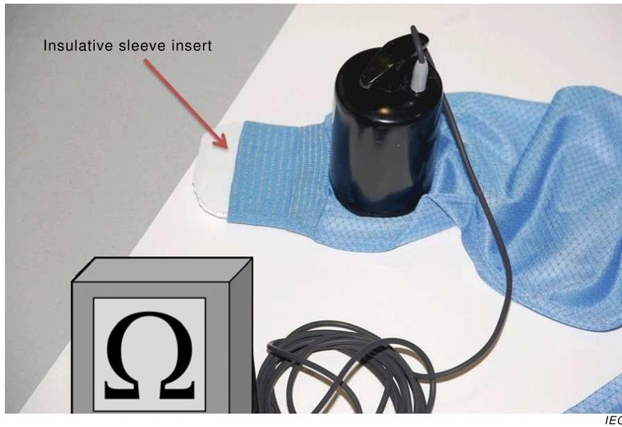
**Figure 2 – Test set-up – Resistance point-to-point
