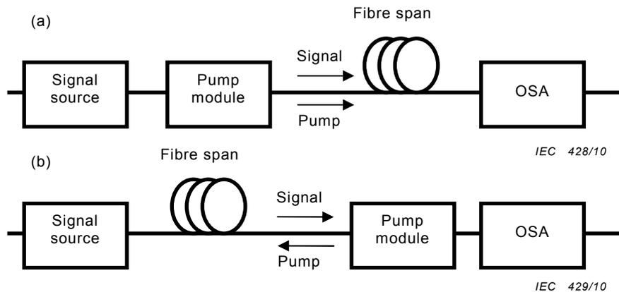
**Figure 9 – Typical configuration used to measure on-off gain (a) for co-propagating DRA and (b) for counter-propagating DRA**
