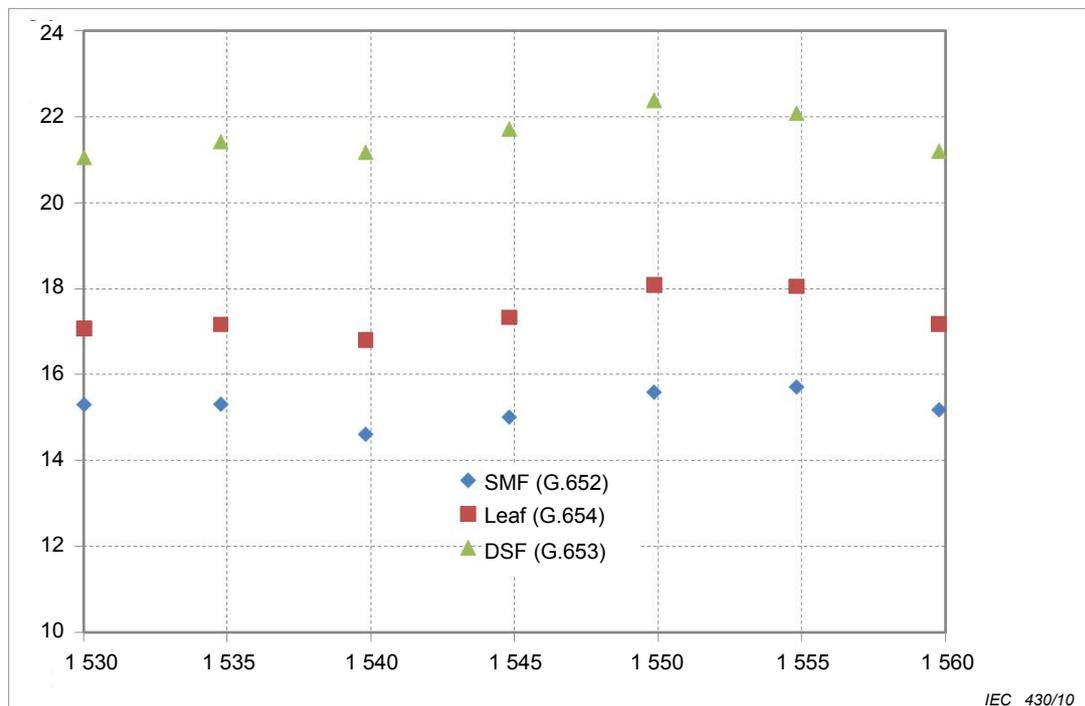
NOTE In each case, 75 km of transmission fibre was used, and the Raman pump were configured as: 290 mW at 1 424 nm, 410 mW at 1 452 nm.
