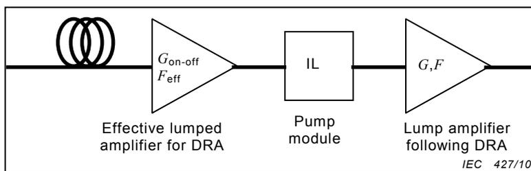
NOTE  $G_{on-off}$  and  $F_{eff}$  are the on-off gain and effective noise figure of the DRA, and  $G, F$  are the gain and NF of a lumped amplifier that would typically follow the Raman pump module.
