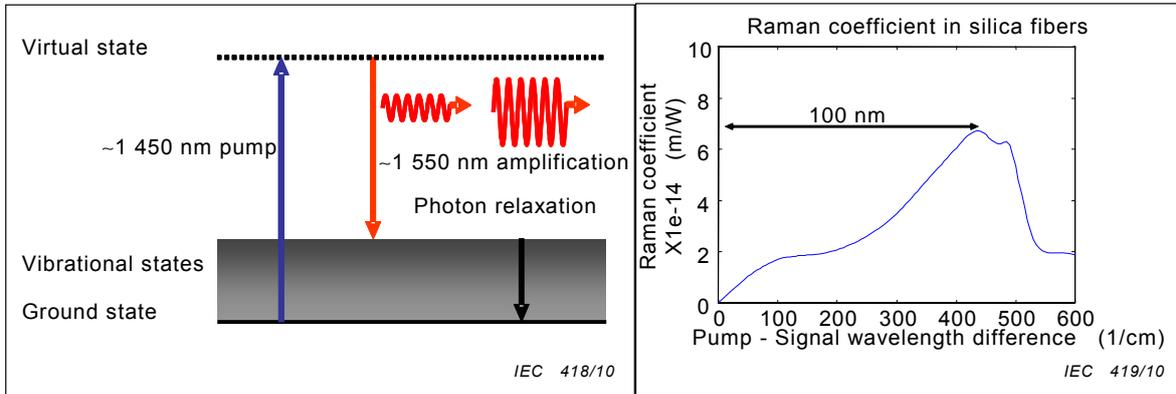
**Figure 1 – Stimulated Raman scattering process (left) and Raman gain spectrum for silica fibres (right)**
