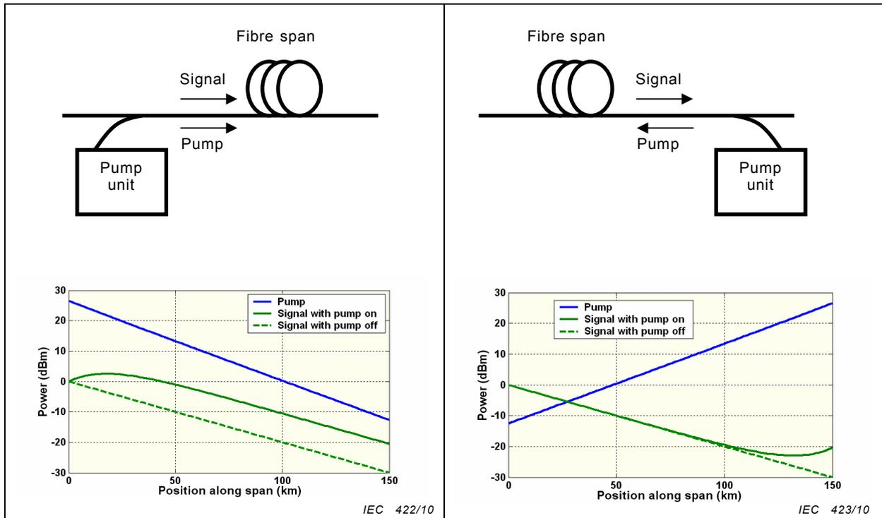
NOTE Two pumps at different wavelength provide a total of 500 mW, resulting in 10 dB on-off gain across the C-band.
