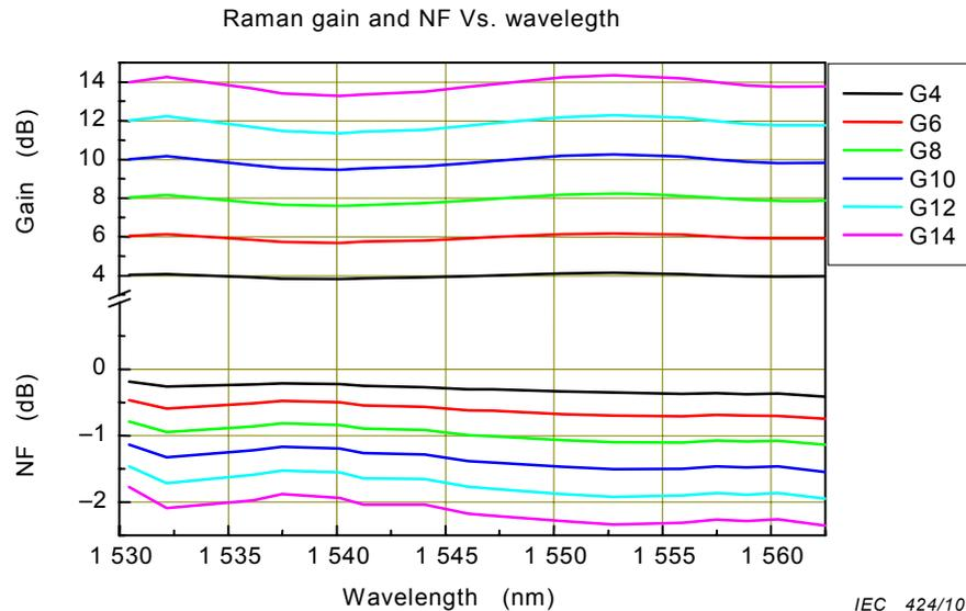
NOTE The various curves correspond to different composite pump powers.
