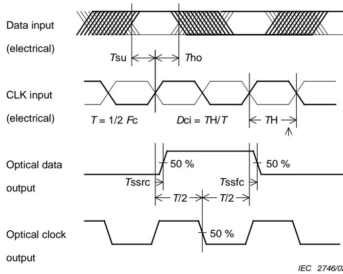
Figure 5 – Definition of transmitter skew
