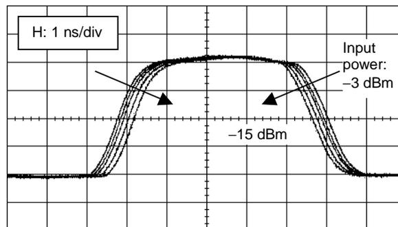
Figure 16 – An example of receiver skew affected by receiving power level
