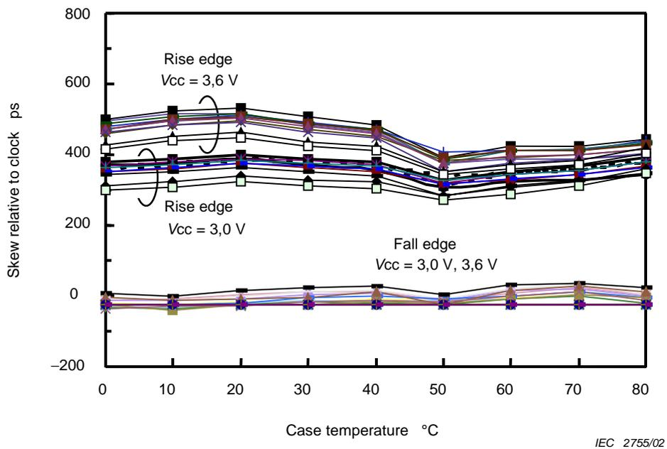
Figure 14 – Temperature dependence of transmitter skew
