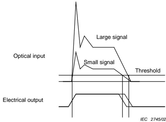
**Figure 4 – Receiver skew from the optical level difference**
