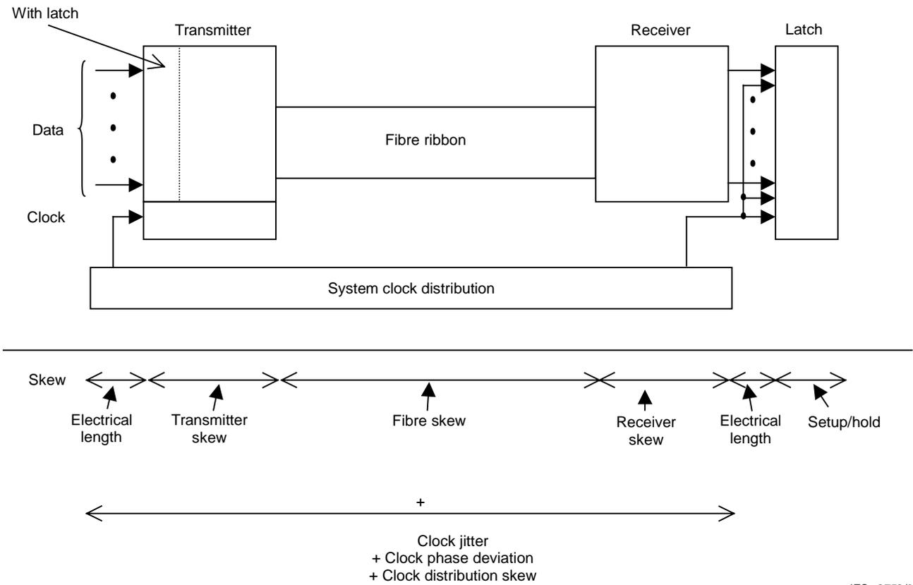
**Figure 11 – System configuration in case of system clock supply**
