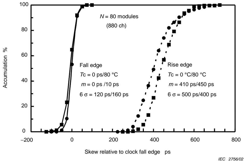
Figure 15 – Accumulation curve of transmitter skew at 0 °C and 80 °C case temperature
