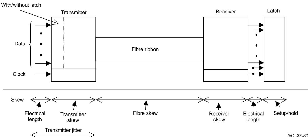
**Figure 7 – System configuration in case of simultaneous clock transmission**
