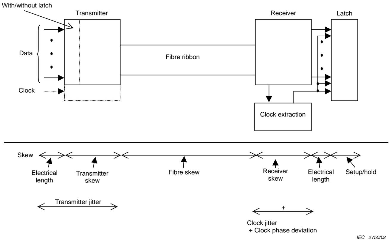
Figure 9 – System configuration in case of clock extraction from the representative port
