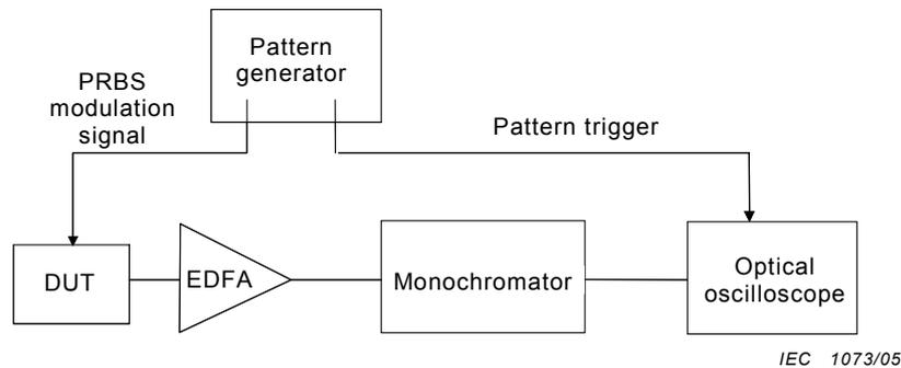
**Figure 8 – Set-up for the monochromator method**
