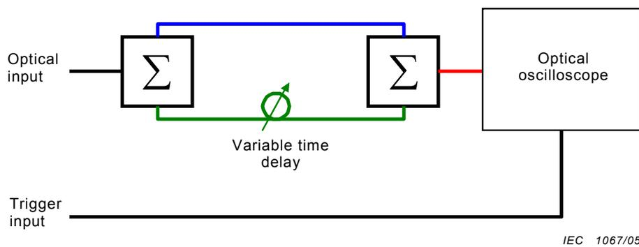
**Figure 2 – Simplified diagram for the frequency discriminator method**
