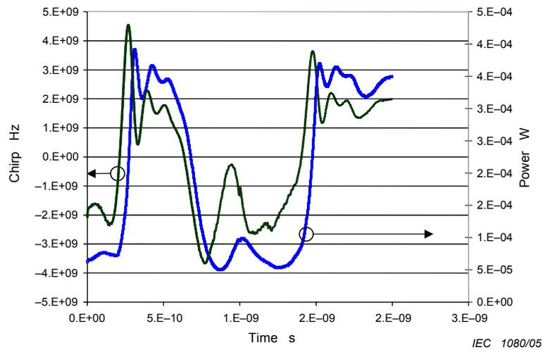
A directly modulated laser has significant transient and adiabatic chirp
