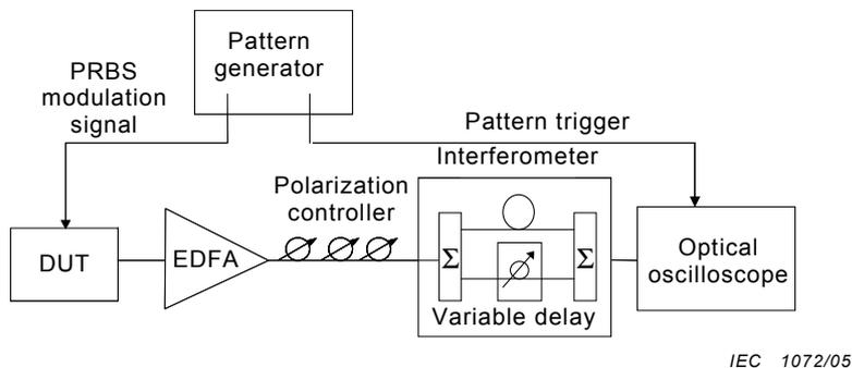
**Figure 7 – Setup for the frequency discriminator method**
