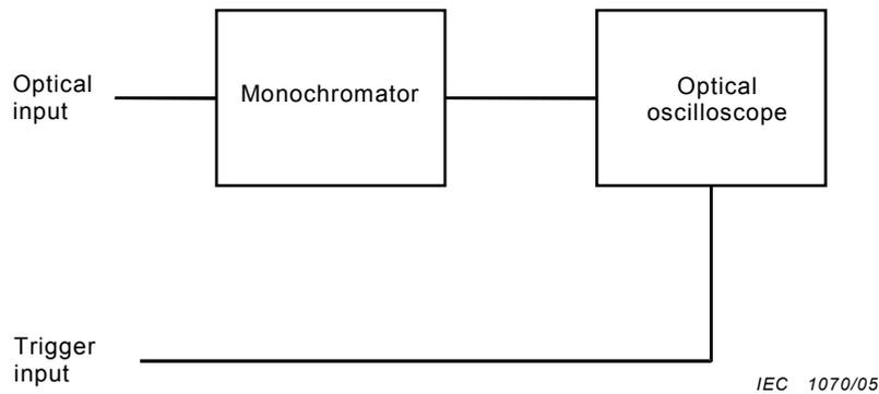
**Figure 5 – Simplified block diagram for the monochromator method**
