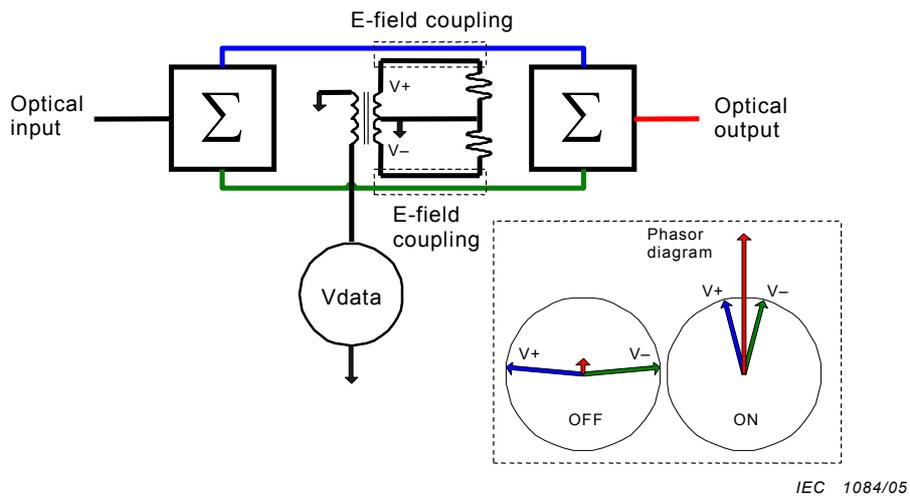
Figure B.6 – Schematic representation of a Mach-Zehnder modulator
