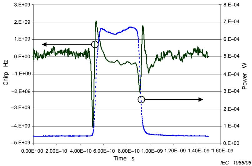
Figure B.7 – Chirp measurement on a Mach-Zehnder modulator showing only transient chirp
