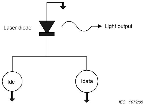
**Figure B.1 – Schematic representation of a directly modulated laser**
