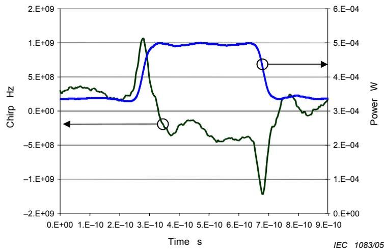
**Figure B.5 – Chirp of an EML with an additional transient characteristic**
