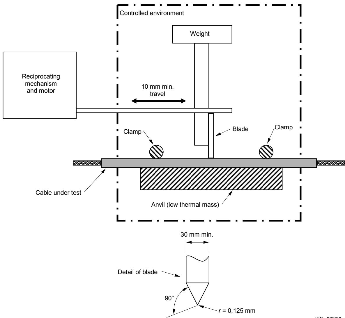
**Figure 1 – Scrape abrasion test equipment and set-up**
