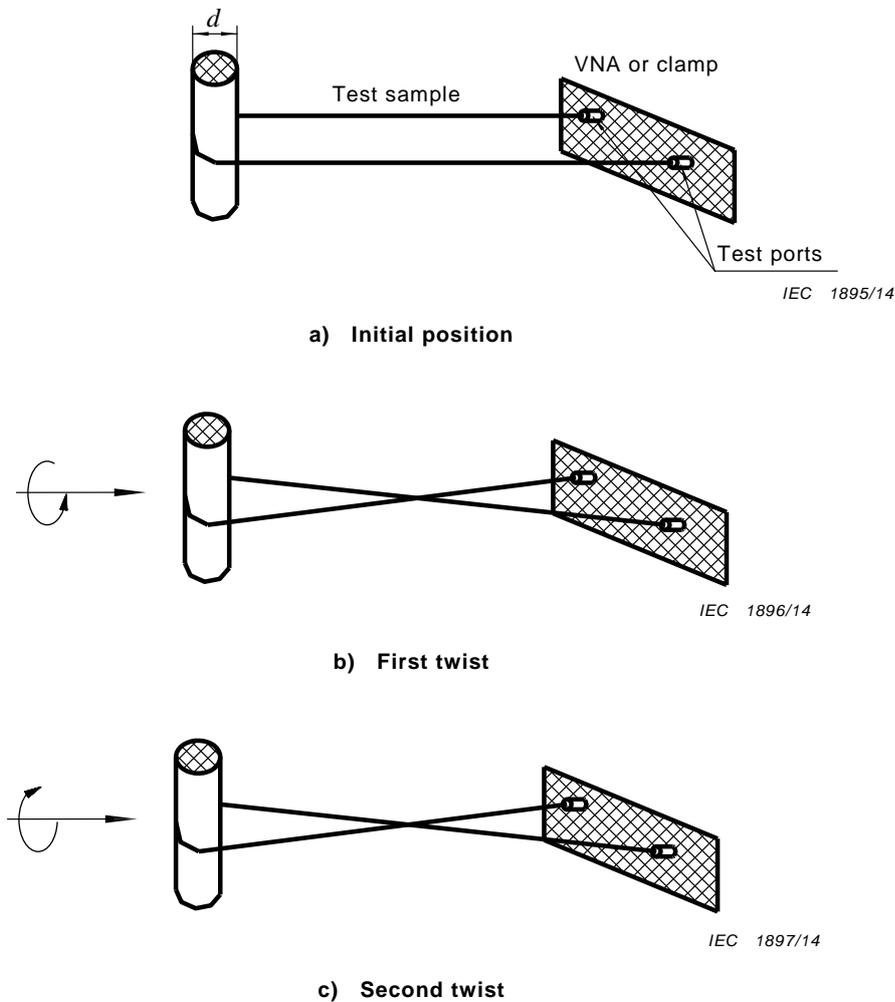
**Figure 8 – Twist test**
