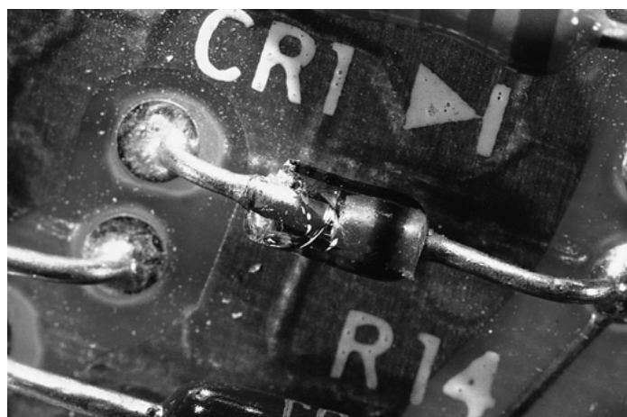
Figure 48 – Damage to axial component with glass body
