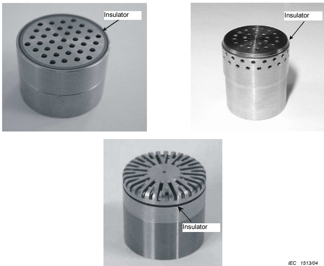
Figure A.3 – Examples of electrostatic actuators forming integral parts of the microphone protection grids
