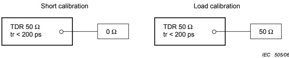
Figure B.1 – Signal pairs impedance setup calibration
