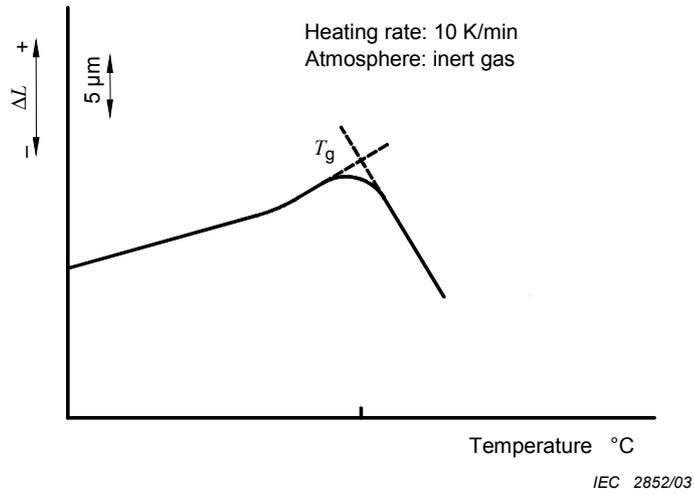
**Figure 3 – Thermomechanical analysis (TMA) (Penetration mode):
