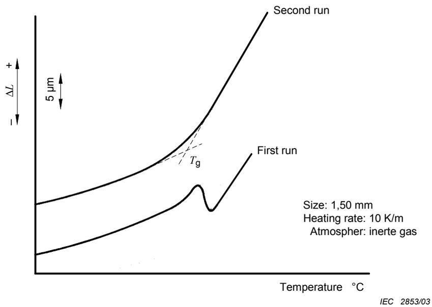
**Figure 4 – Thermomechanical analysis (TMA) (Expansion mode):
