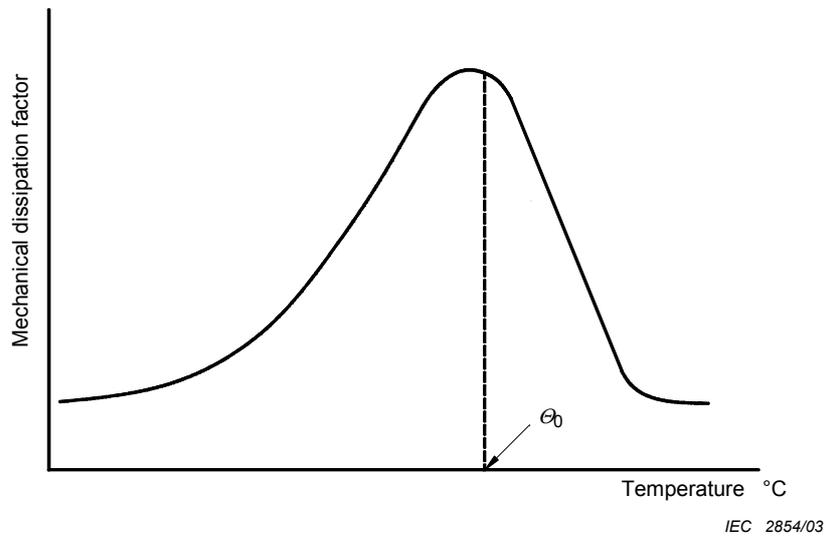
Figure 5 – Typical mechanical dissipation factor profile
