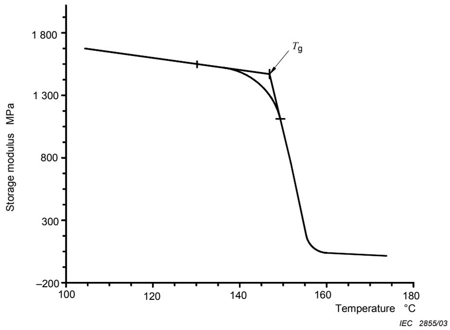
Figure 6 – Dynamic mechanical analysis (DMA):
