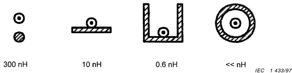
NOTE – Typical values for the  $Z_t$  at HF are given as mutual inductance  $M$  in nH/m. The values of the HF  $Z_t$  depend on the shape rather than on the total cross-section of the PEC.
