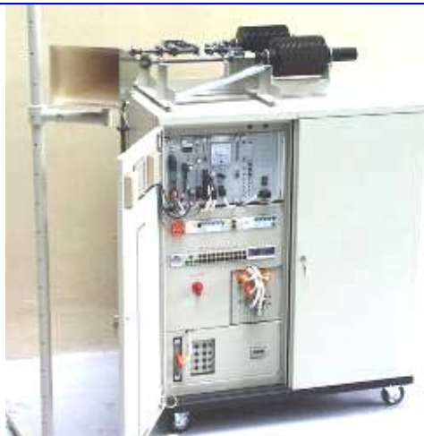
HPM generator 9 GHz with antenna 3 dB beam angle = 10^\circ
