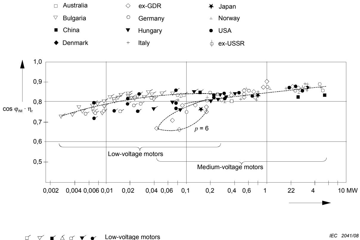
**Figure 14 – Product  $\cos \varphi_{rM} \times \eta_{rM}$  of low-voltage and medium-voltage motors, 50 Hz and 60 Hz**
