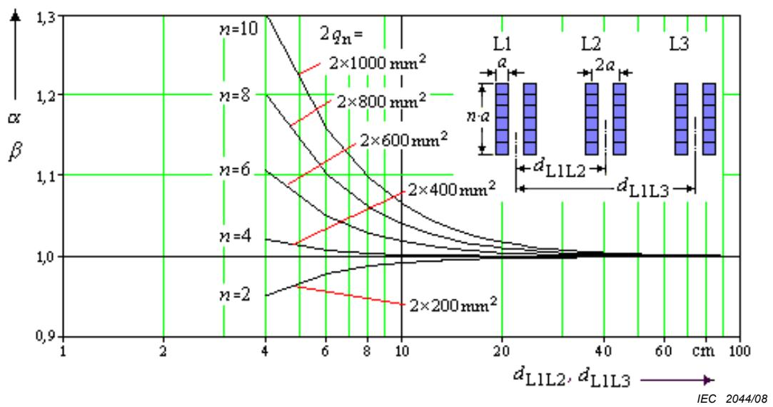
b) For two bars per main conductor;  $a = 10$  mm
