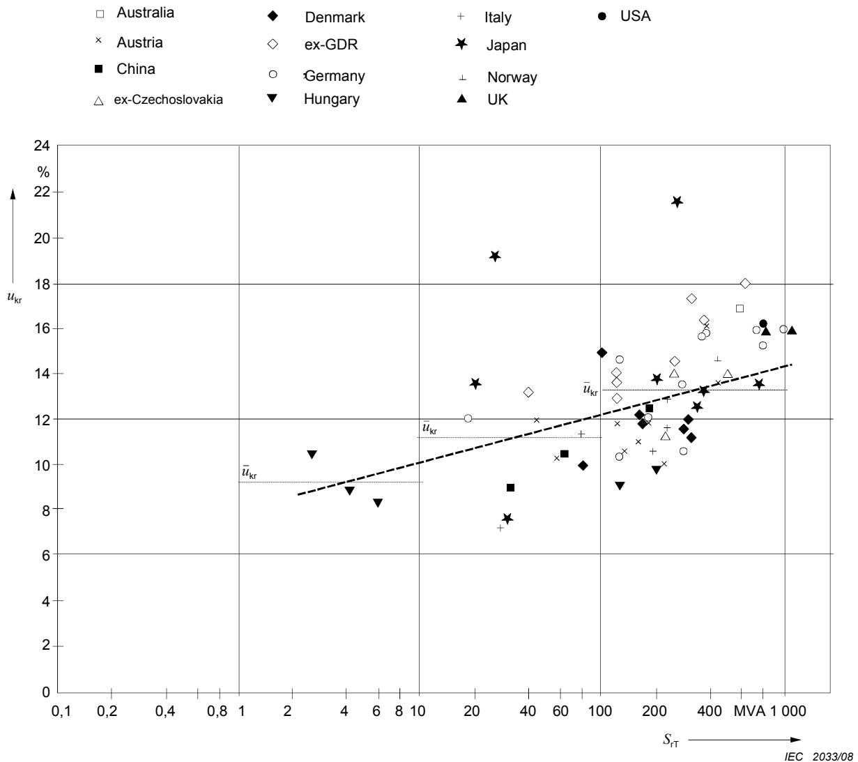
**Figure 6 – Rated short-circuit voltages  $u_{kr}$  of network transformers**
