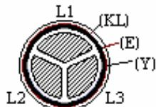
Belted cable with three copper or aluminium (A) conductors, a mass-impregnated paper insulation for conductors (and belt), a smooth extruded aluminium sheath (KL), protective covering with an embedded layer of elastomer tape or plastic film (E) and a sheath of thermoplastic material based on PVC (Y): N(A)KLEY
