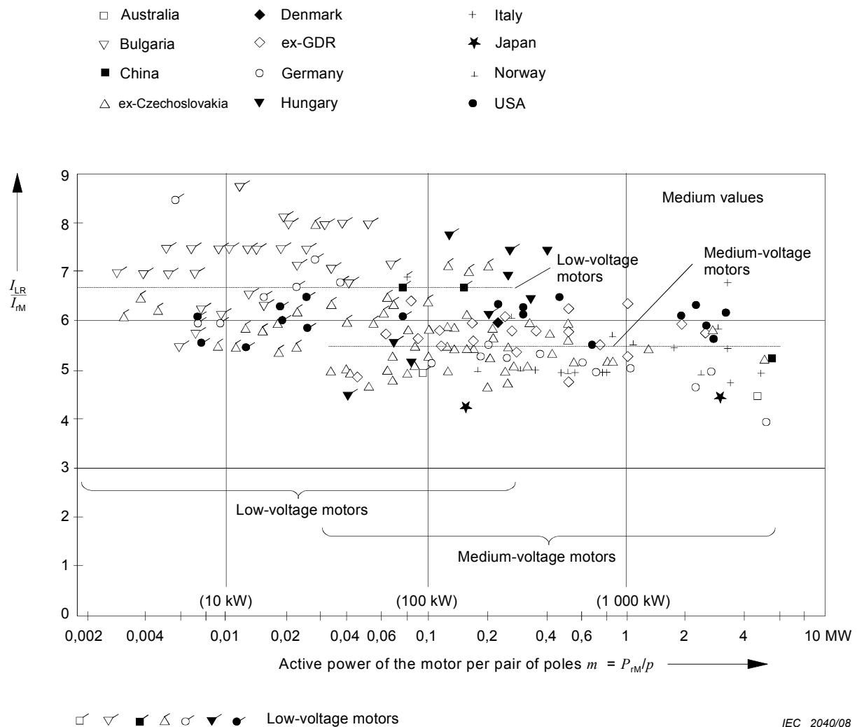
**Figure 13 – Ratio  $I_{LR}/I_{RM}$  of low-voltage and medium-voltage asynchronous motors, 50 Hz and 60 Hz**
