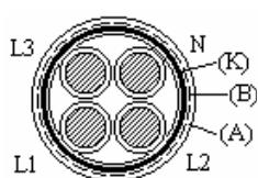
Cable with four (or three and a half) copper or aluminium (A) conductors, a mass-impregnated paper insulation for conductors (and belt), lead sheath (K) with steel tape armouring (B) and an outer serving of fibrous material (A): N(A)KBA
