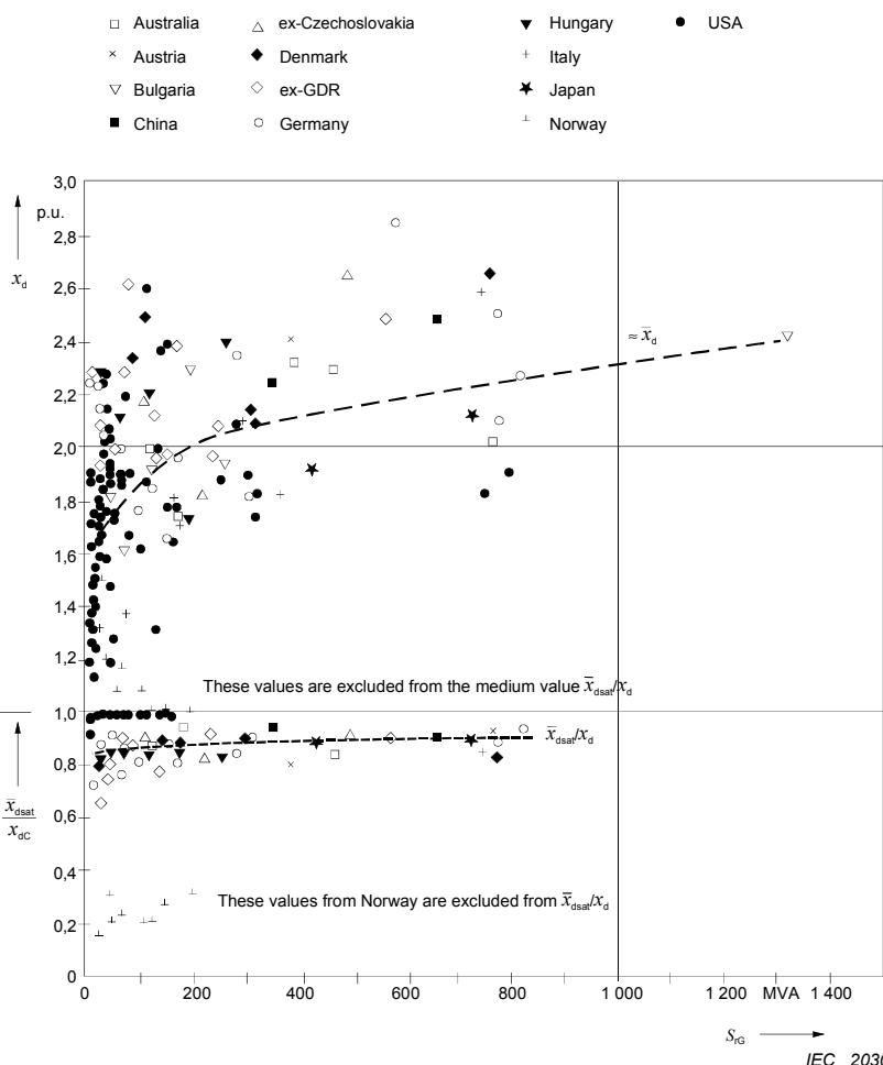
**Figure 3 – Unsaturated and saturated synchronous reactance of two-pole turbo generators 50 Hz and 60 Hz (relative values)**
