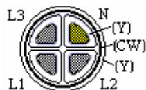
Cable with four or three copper or aluminium (A) conductors, insulation of thermoplastic material based on PVC (Y), concentric copper conductor, helically applied (CW), and a sheath of thermoplastic material based on PVC (Y): N(A)YC(WY)
