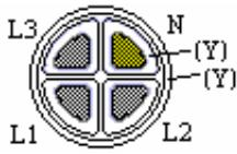
Cable with copper or aluminium (A) conductors (example: four-core cable), insulation of thermoplastic material based on PVC (Y) and a protective covering in the form of a sheath of thermoplastic material based on PVC (Y): N(A)YY
