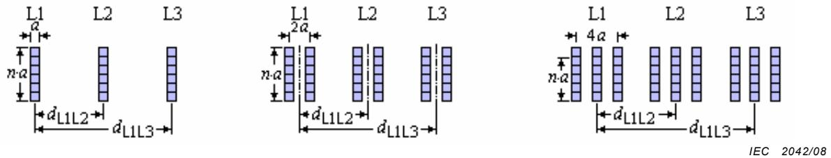
$$g_{L1L1} = (0,23 + 0,2225 \times n) \times a \quad g_{L1L1} = (0,74 + 0,2265 \times n) \times a \quad g_{L1L1} = (1,218 + 0,2275 \times n) \times a$$
