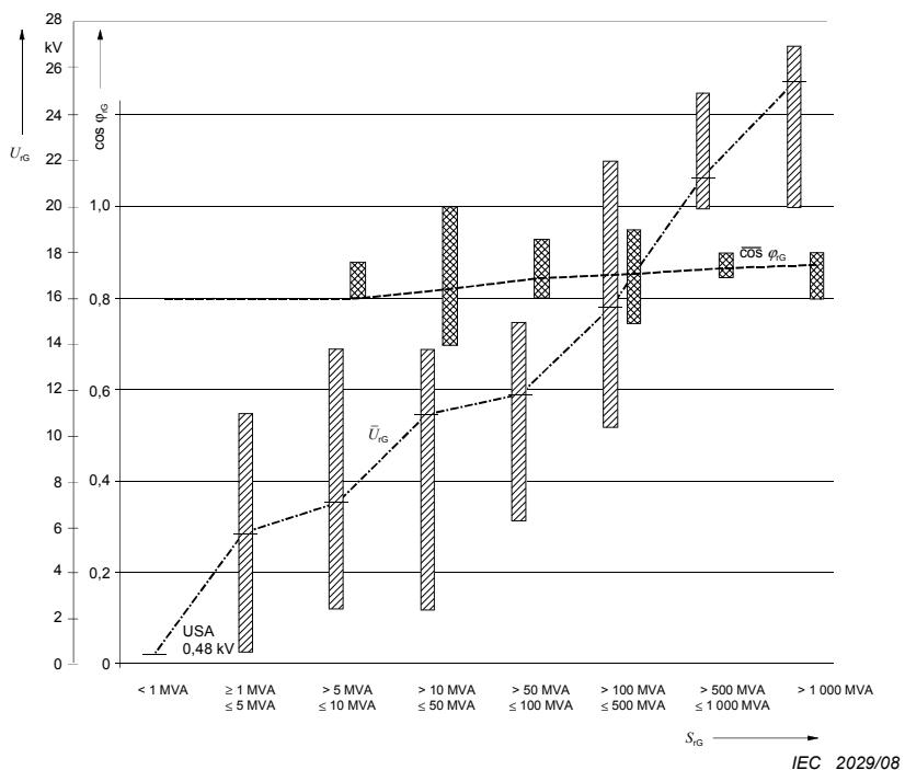
**Figure 2 – Rated Voltage  $U_{rG}$  and rated power factor  $\cos\varphi_{rG}$  of synchronous machines (Turbo generators, salient pole generators, motors and condensers 50 Hz and 60 Hz)**
