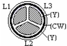
**Cable with four conductors NYC(WY):**
