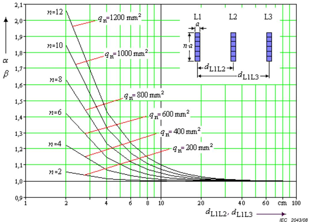
a) For one bar per main conductor;  $a = 10 \text{ mm}$
