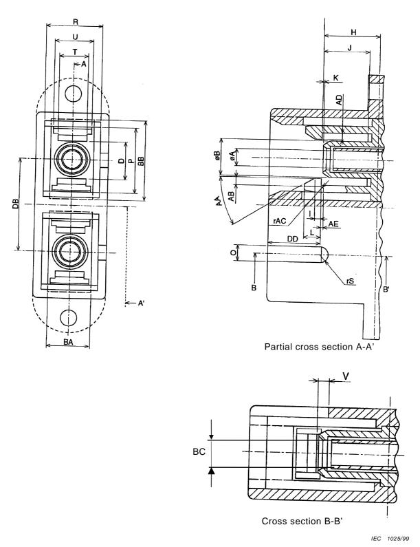
NOTE – The dotted lines are for information only and represent the outer shape of the fixture of the adaptor.
