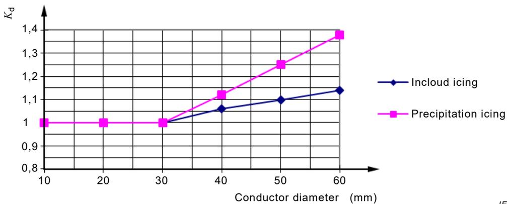
**Figure 11 – Factor  $K_d$  related to the conductor diameter**
