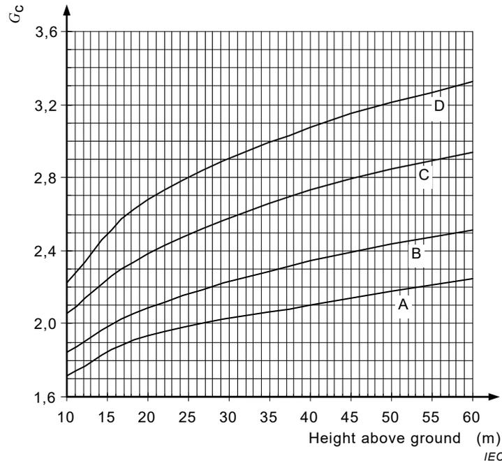
**Figure 4 – Combined wind factor  $G_c$  for conductors for various terrain categories and heights above ground**
