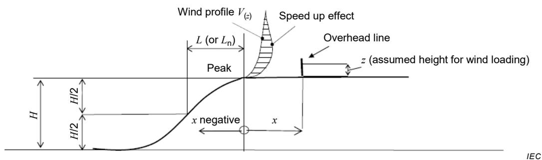
**Figure G.1 – Diagram of typical topographical cross-section**
