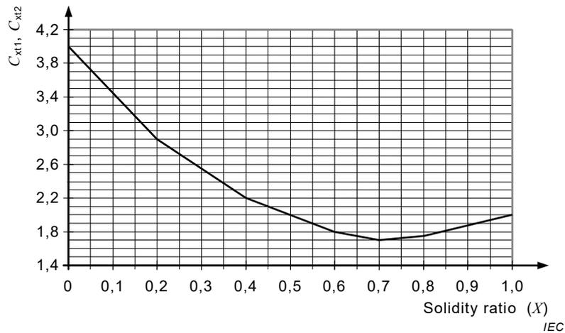
Figure 8 – Drag coefficient  $C_{xt}$  for lattice supports made of flat sided members
