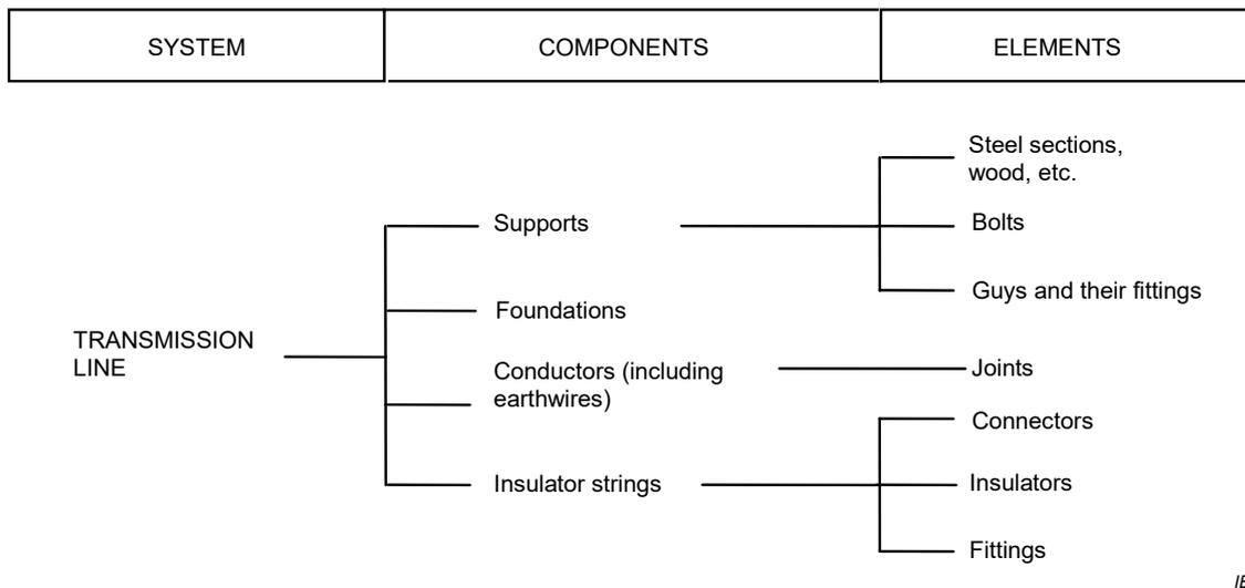
**Figure 1 – Diagram of a transmission line**
