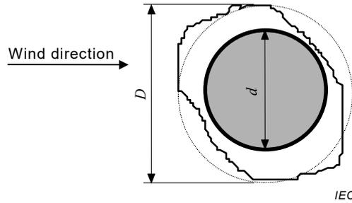
**Figure 14 – Equivalent cylindrical shape of ice deposit**
