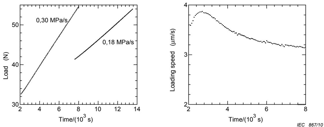
Figure C.2 – Time variation of load and loading speed
