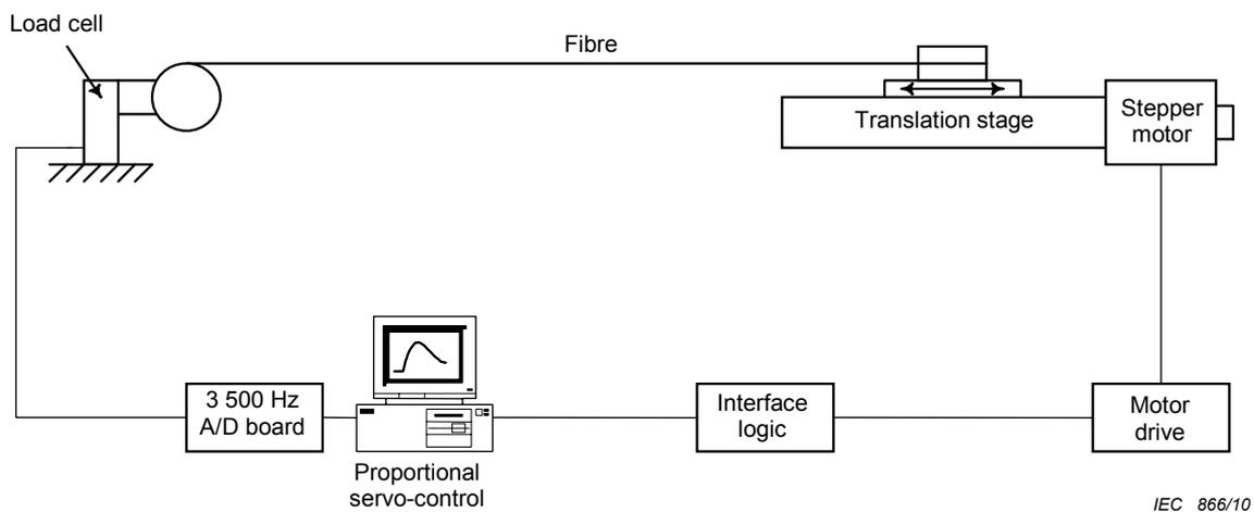
Figure C.1 – System to control stress rate
