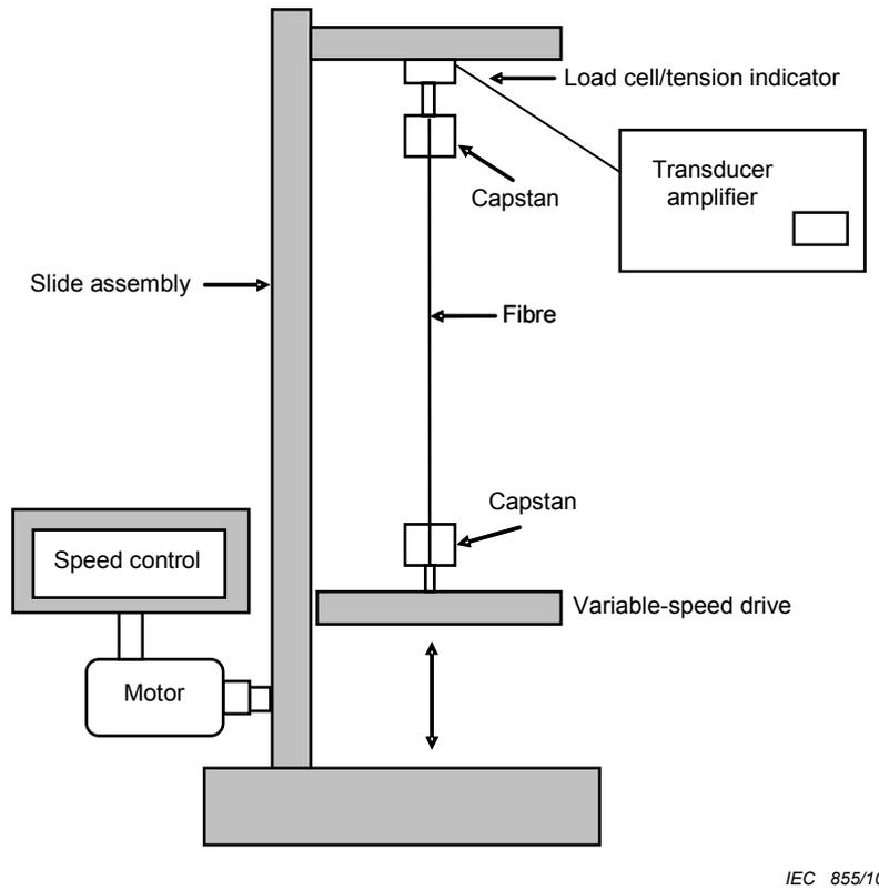
**Figure A.2 – Translation test apparatus**
