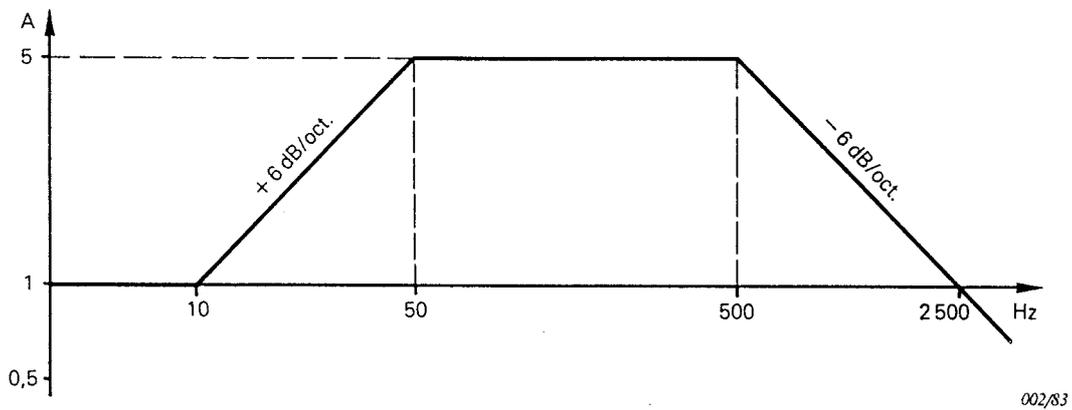
The weighting curve is based on a horizontal flywheel of the television receiver having a minimum gain of 16 000, a resonant frequency of 160 Hz and a damping factor 1,6.
