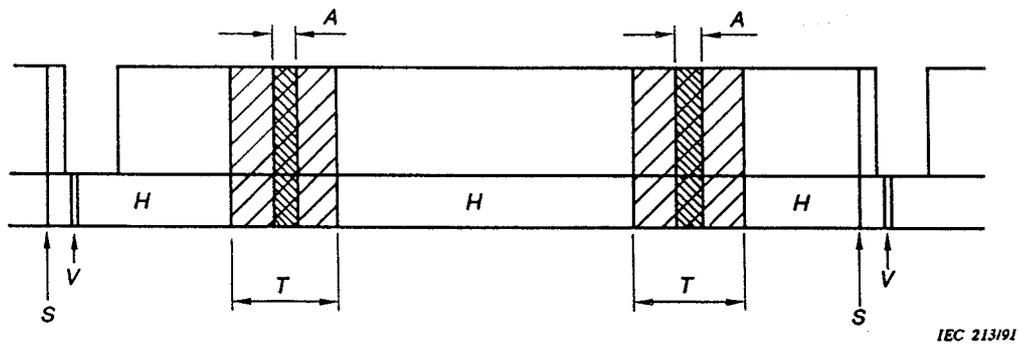
Figure 1 - Signal transition (one field) - One head is used per scan (see 6.1.2 a))
