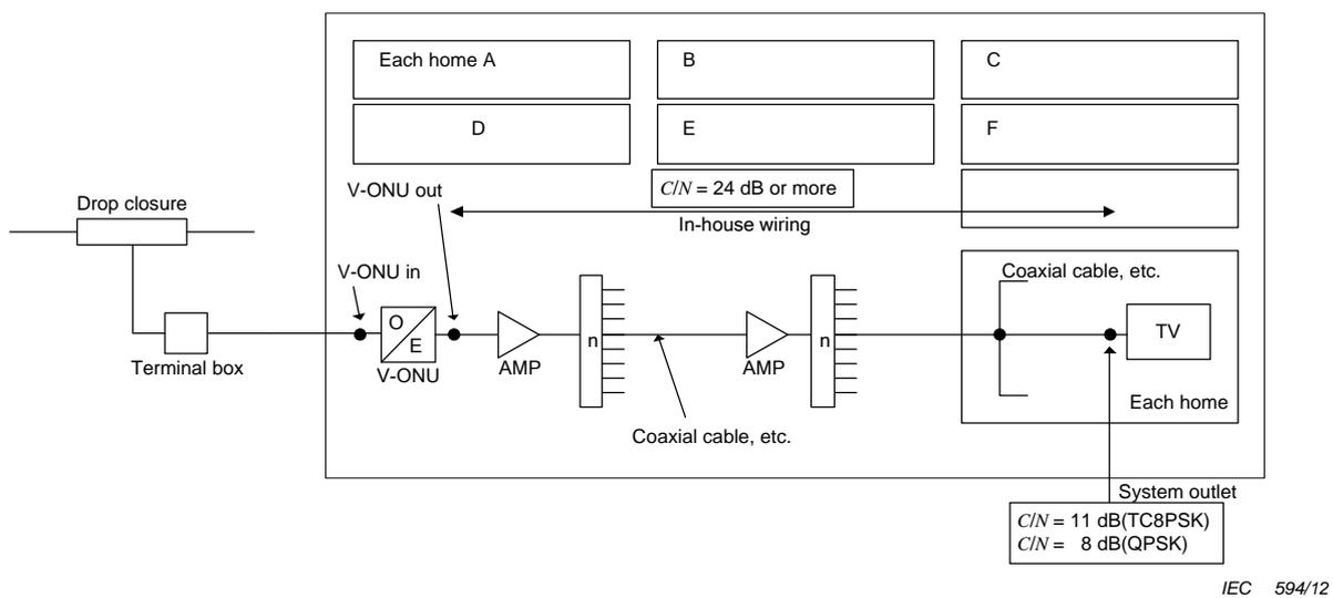
Figure 11 – Section of *C/N* ratio specification (24 dB) for in-building wiring (in case of coaxial cable distribution after V-ONU)
