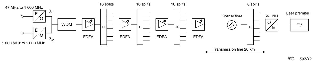
**Figure A.3 – Example of a multi-channel with CS supplementary service system of 2 000 terminals**
