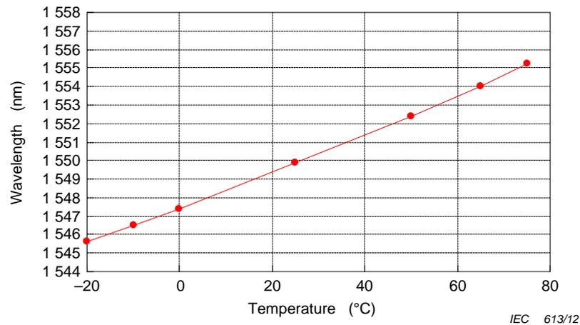
**Figure C.3 – Wavelength variation of CWDM transmitter against ambient temperature**
