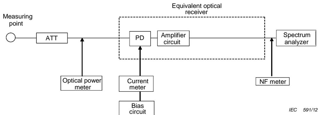
**Figure 8 – *RIN* measurement setup**
