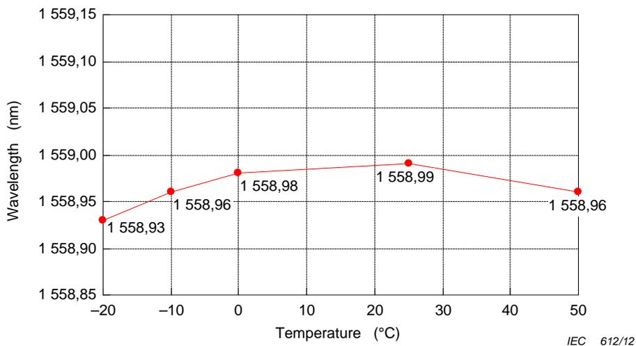
Figure C.2 – Wavelength variation of DWDM transmitter against ambient temperature
