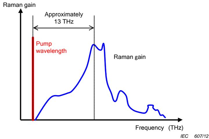
Figure B.2 – Wavelength dependency of Raman crosstalk
