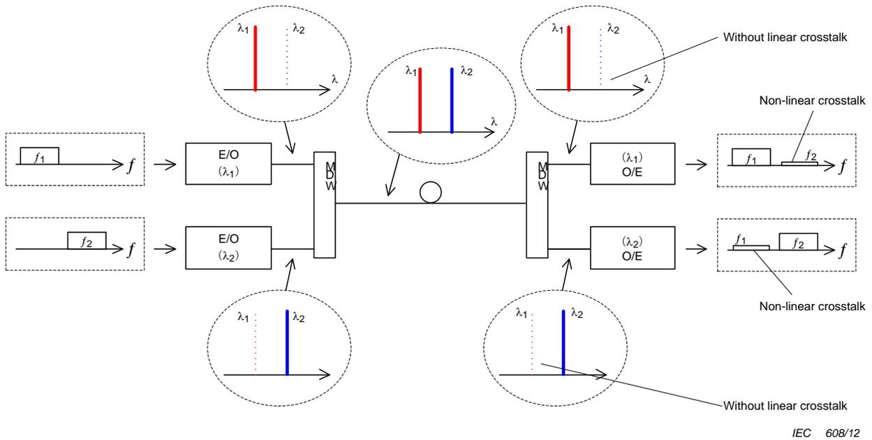
Figure B.3 – Nonlinear crosstalk between two wavelengths
