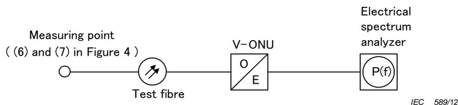
**Figure 6 – Measurement of carrier level and carrier-to-noise ratio**
