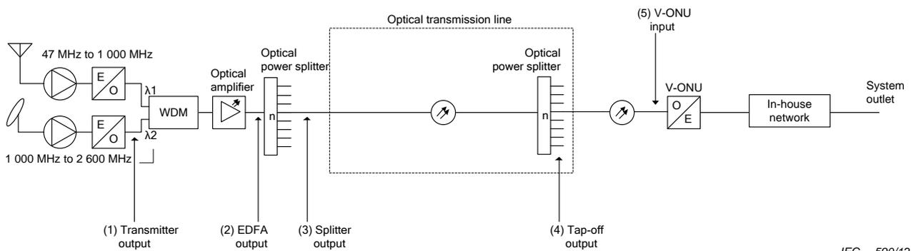
Figure 7 – Measuring points in a typical FTTH system
