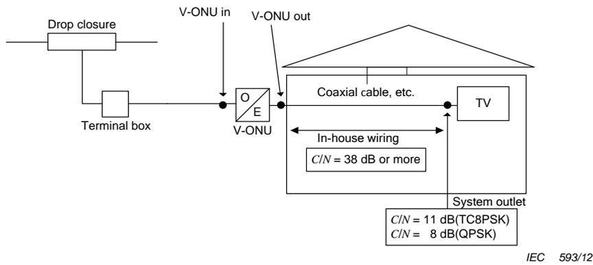
Figure 10 – Section of *C/N* ratio specification (38 dB) for in-house wiring
