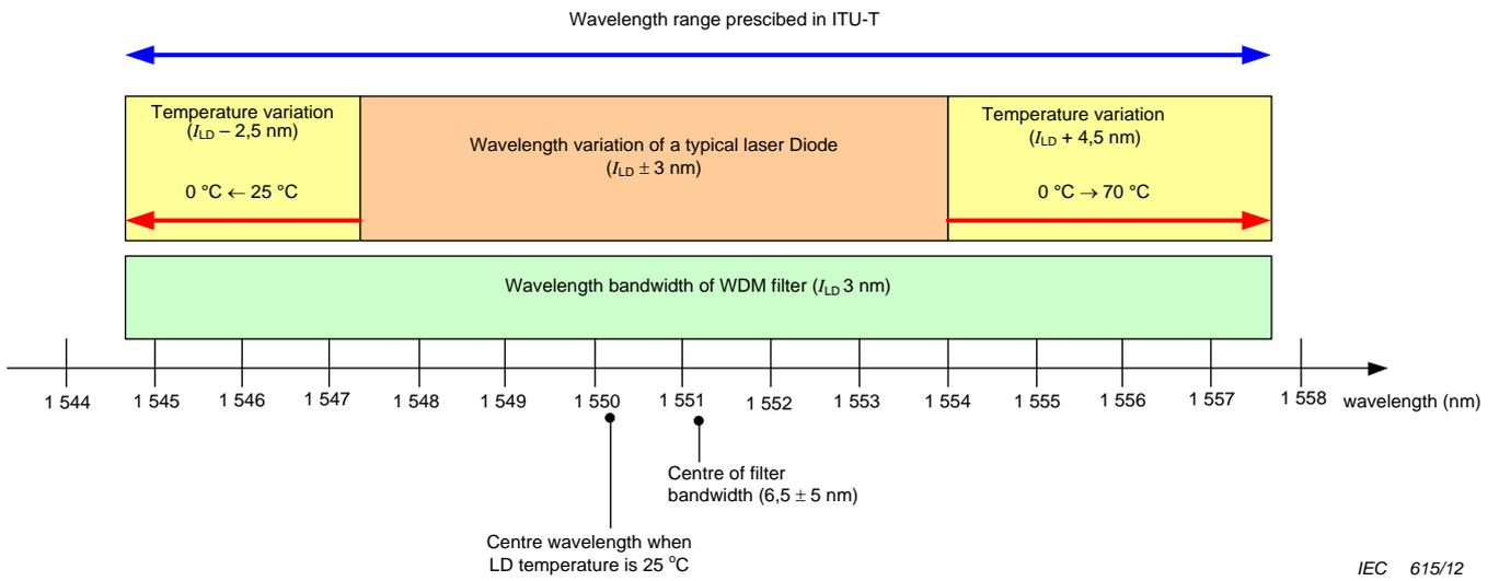
Figure C.5 – Example of CWDM filter design
