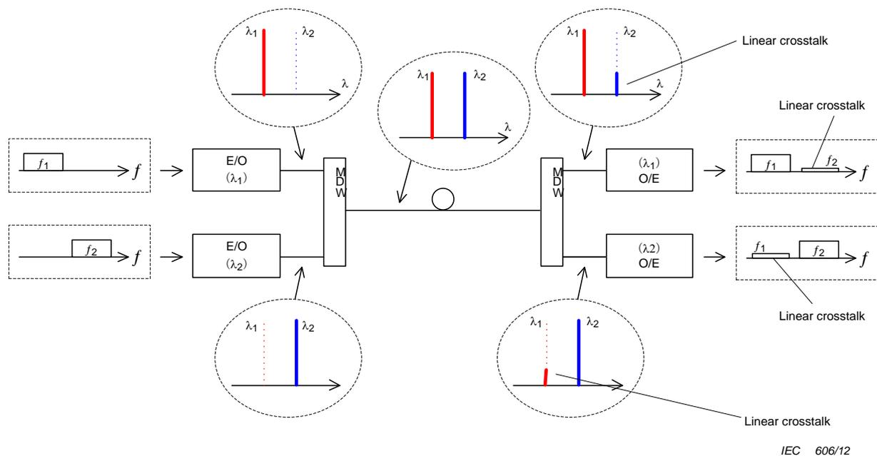
**Figure B.1 – Linear crosstalk between two wavelengths**
