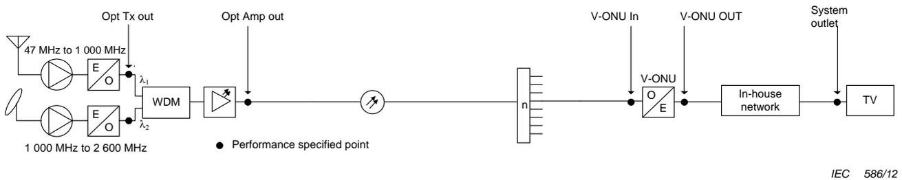
**Figure 3 – Performance specified points of the optical system**
