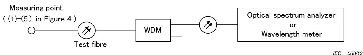
**Figure 5 – Measurement of optical wavelength using WDM coupler**
