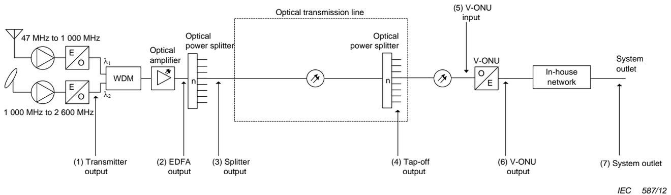
**Figure 4 – Measuring points in a typical video distribution system**
