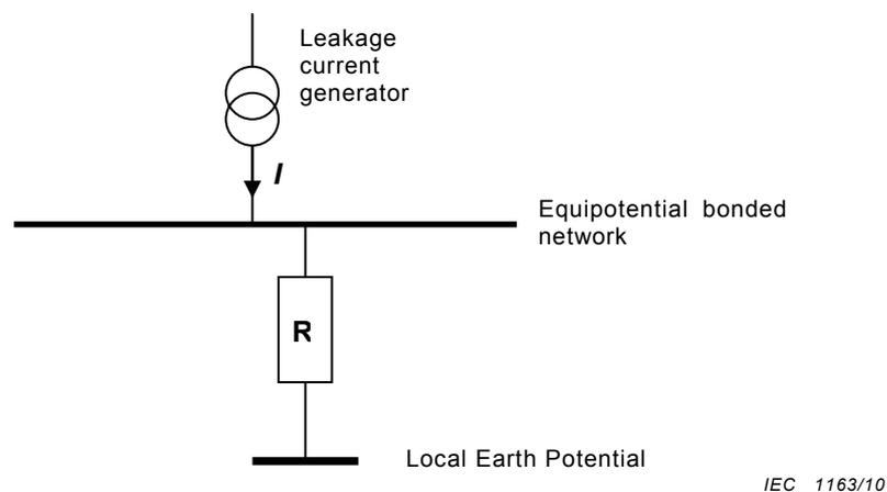
**Figure A.1 – Systematic of earth loop resistance**
