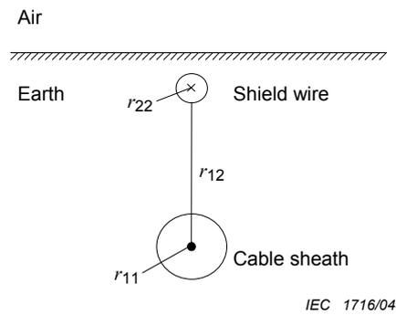
**Figure B.1 – Principle of single shield wire**
