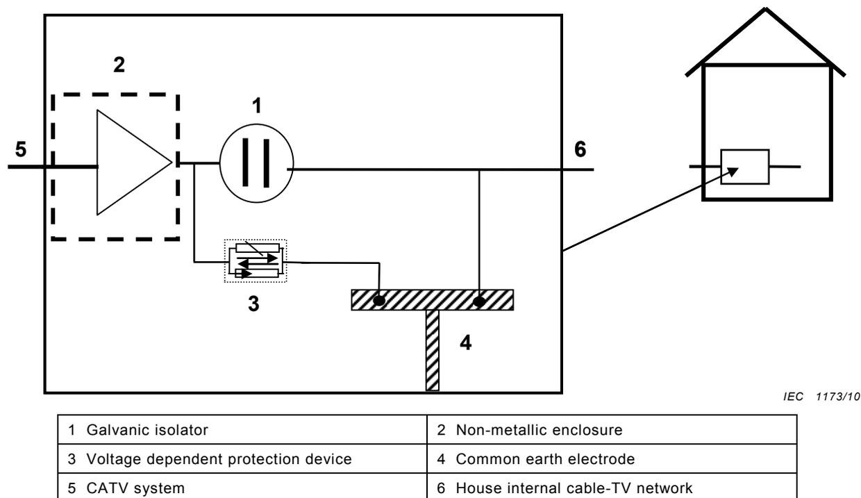
**Figure D.8 – Example of an installation placing the amplifier in front of the galvanic isolator**
