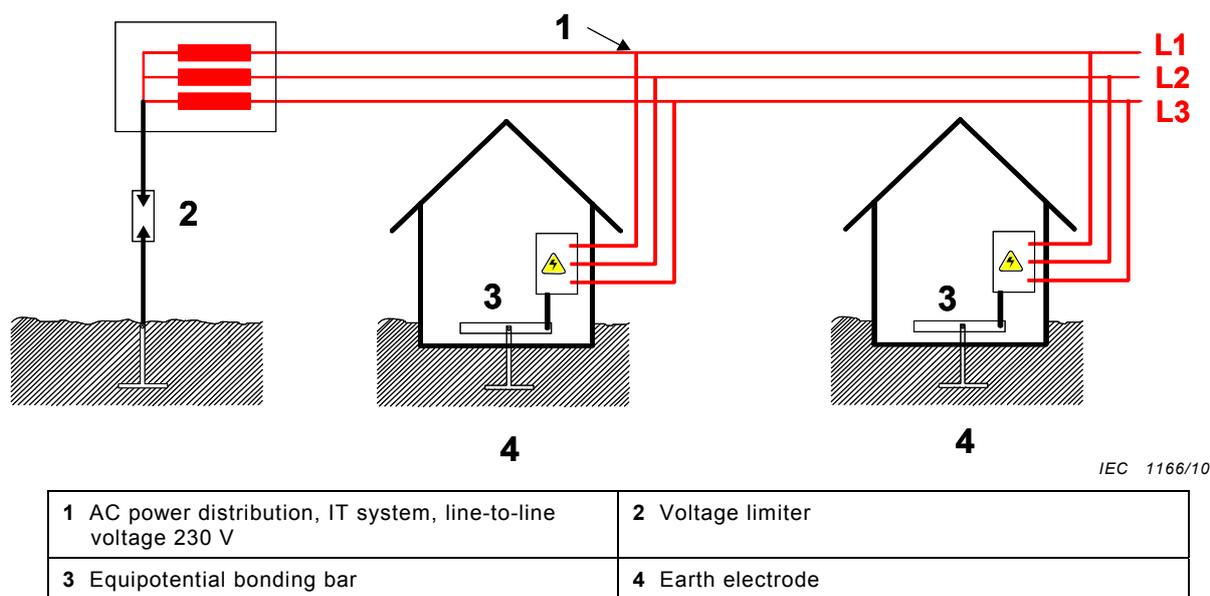
**Figure D.1 – IT power distribution system in Norway**
