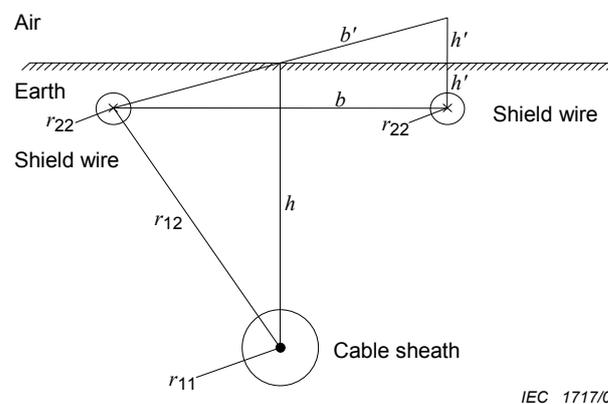
**Figure B.2 – Principle of two shield wires**
