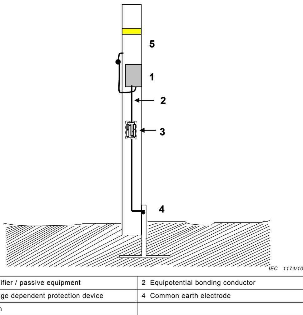
**Figure D.9 – Example of protection using a voltage depending device on network installations on poles**
