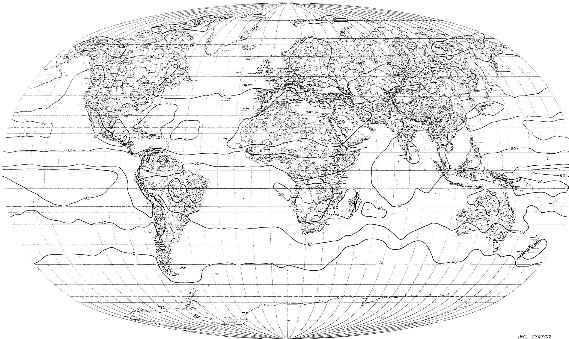
Figure A.1 – Mean relative global irradiation for the month of June (in percent)
