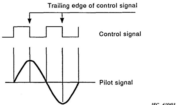
13.1.4.4 Recording level shall be  $36 \text{ dB} \pm 3 \text{ dB}$  below the recorded reference audio level,  $100 \text{ nWb/m} \pm 10 \text{ nWb/m}$  r.m.s. at  $1000 \text{ Hz}$ , in reproducing with time constants of  $t_1 = 50 \mu\text{s}$  and  $t_2 = 3180 \mu\text{s}$ .
