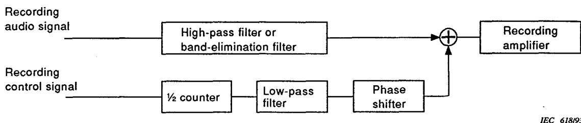
Block diagram of noise-reduction pilot-signal recording
