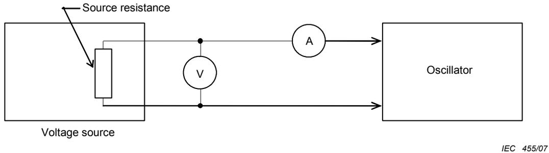
Figure 10 – Test circuit for voltage proof test
