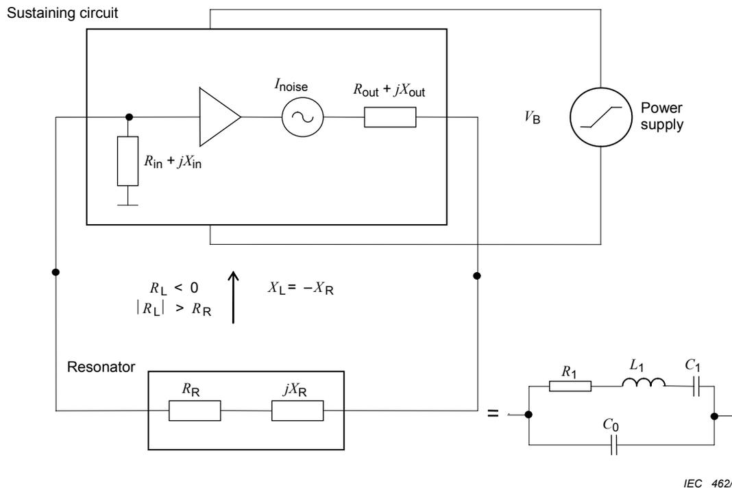
Figure 17 – Generalized oscillator circuit
