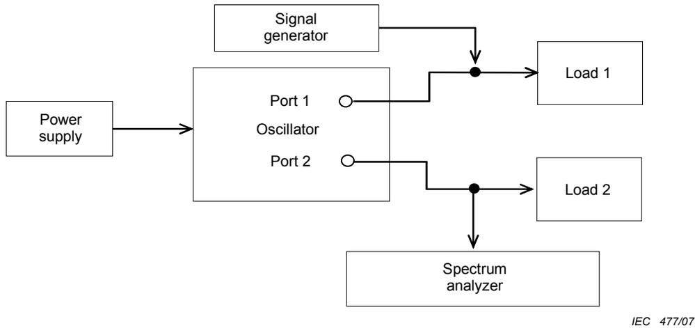
Figure 29 – Test circuit for the determination of isolation between output ports
