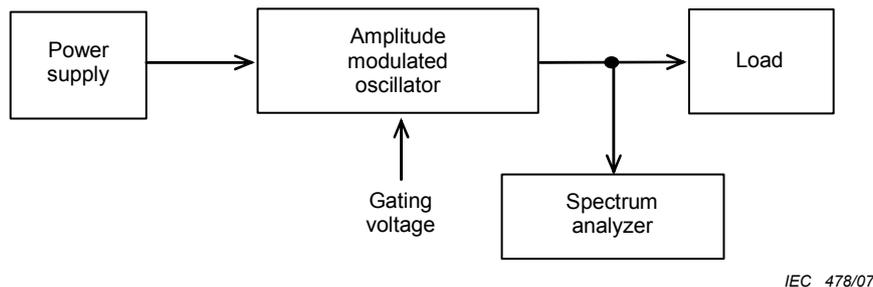
Figure 30 – Test circuit for measuring suppression of gated oscillators
