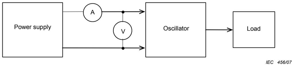
Figure 11 – Test circuit for oscillator input power measurement
