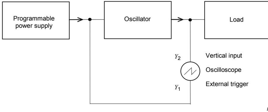
**Figure 18 – Test circuit for start-up behaviour and start-up time measurement**
