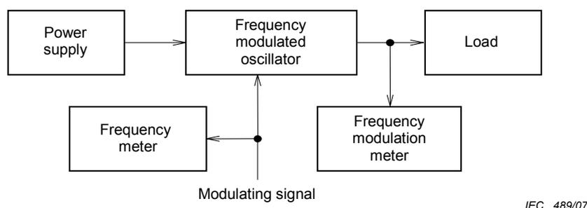
**Figure 41 – Test circuit for the measurement of f.m. deviation**
