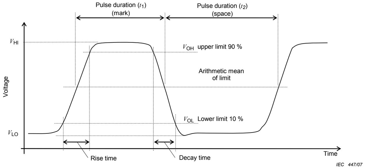
**Figure 3 – Characteristics of an output waveform**
