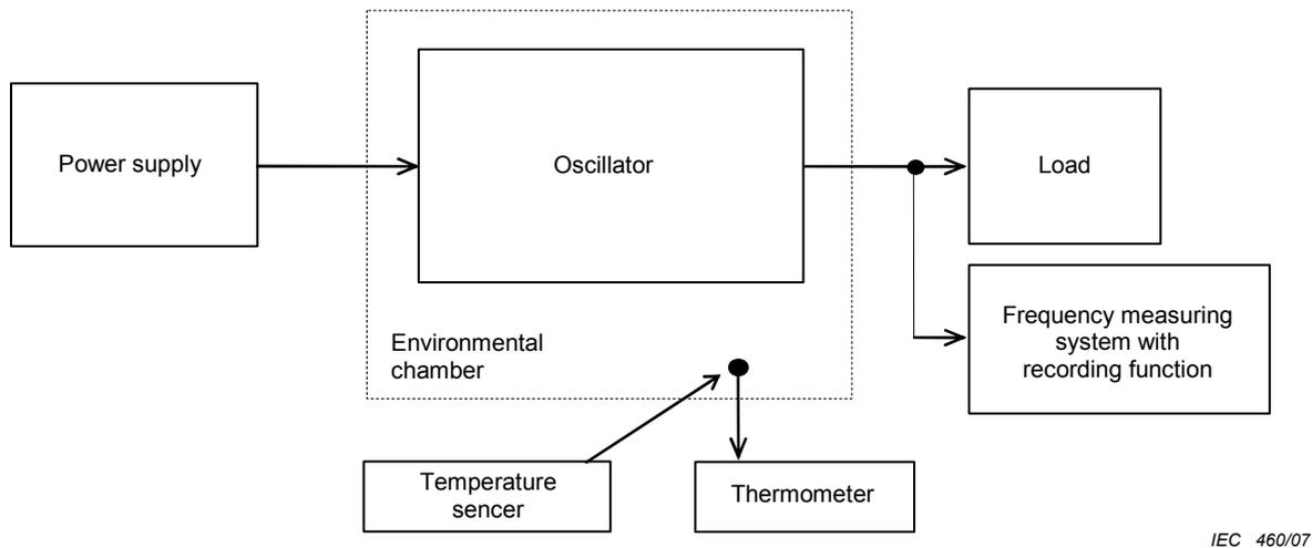
**Figure 15 – Test circuit for measurement of frequency/temperature characteristics**
