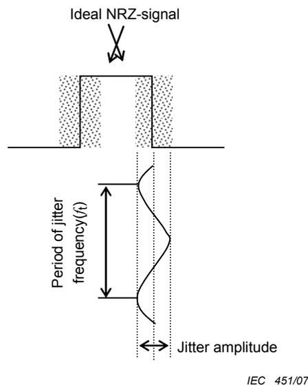
Figure 7 – Jitter amplitude and period of jitter frequency
