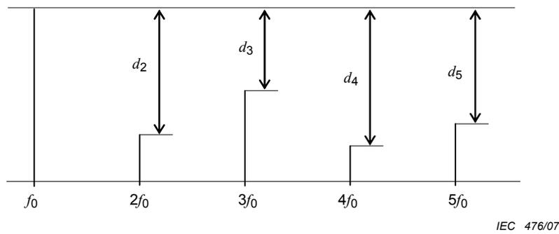
**Figure 28b – Spectrum showing severe harmonic distortion**
