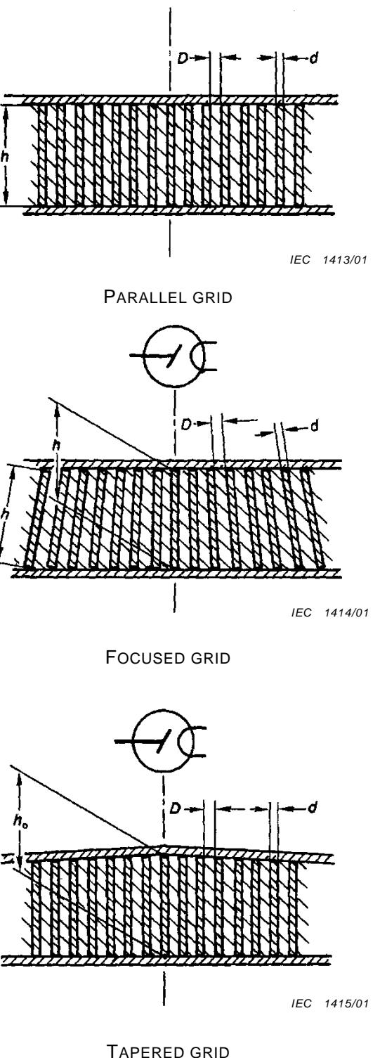
**Figure 1 – Structure of ANTI-SCATTER GRIDS**
