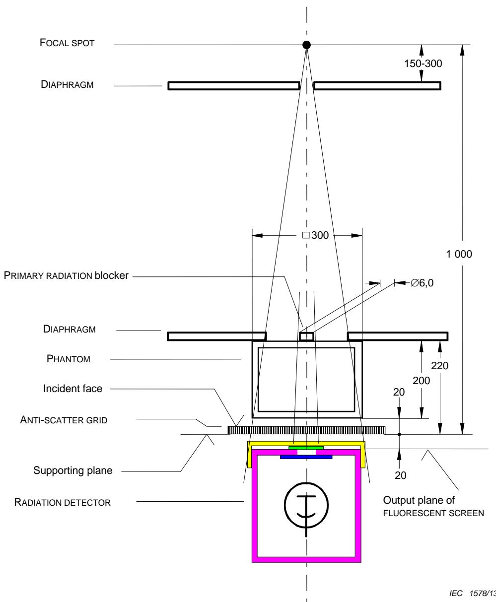
**Figure 4 – Measurement arrangement for general-purpose ANTI-SCATTER GRIDS with BROAD BEAM CONDITION (determination of the TRANSMISSION OF SCATTERED RADIATION)**
