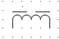
Name: Inductor with gap in magnetic core
