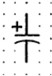
Name: Polarized capacitor, for example electrolytic
