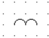
Name: Winding of machine (different functions: commutating or compensating)
