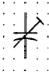
Name: Capacitor with the preset adjustment
