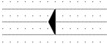
Name: Gas insulated enclosure - partition between two compartments
