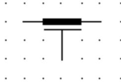
Name: Capacitor, lead-through; Capacitor, feed-through
