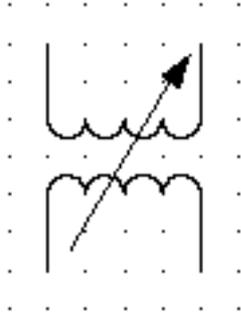
Name: Transformer with variable coupling
