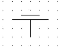
Name: Junction not interrupting the conductor
