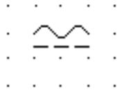
Name: Rectified current with alternating component
