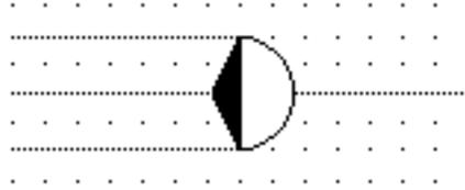
**Name:** Gas insulated conductor - boundary with transformer or reactor bushing
