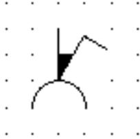
Name: Socket outlet (power) with interlocked switch
