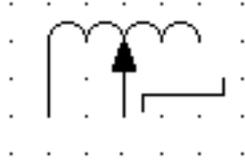
Name: Inductor with moveable contact, variable in steps
