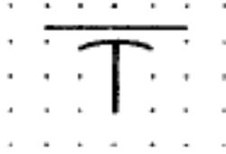
Name: Lead-through capacitor; Feed-through capacitor
