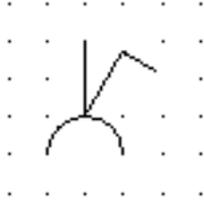
Name: Socket outlet (power) with single-pole switch
