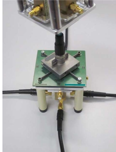
Figure 14 – Measurement of IL and FEXT on the DUT
