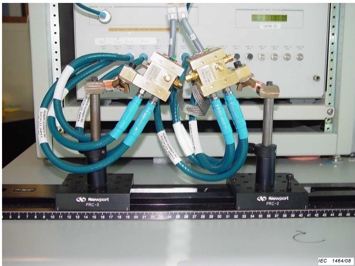
Figure B.3 – Example of fixture, in which balun clusters can slide left and right
