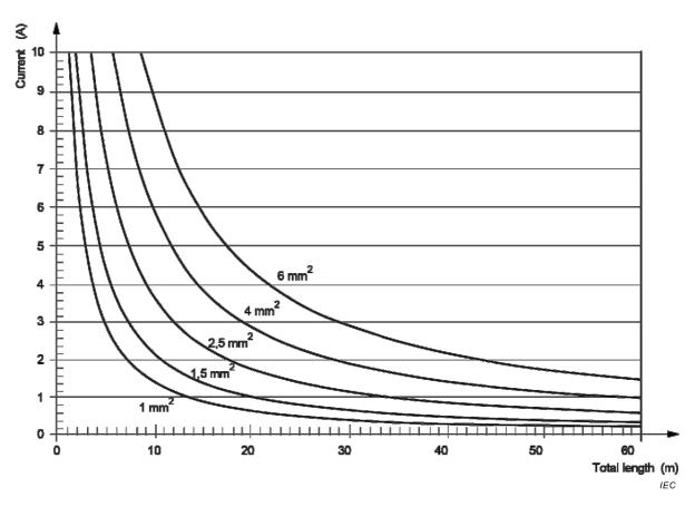
Total length of both cables (positive and negative), in m (route length is half above length)
