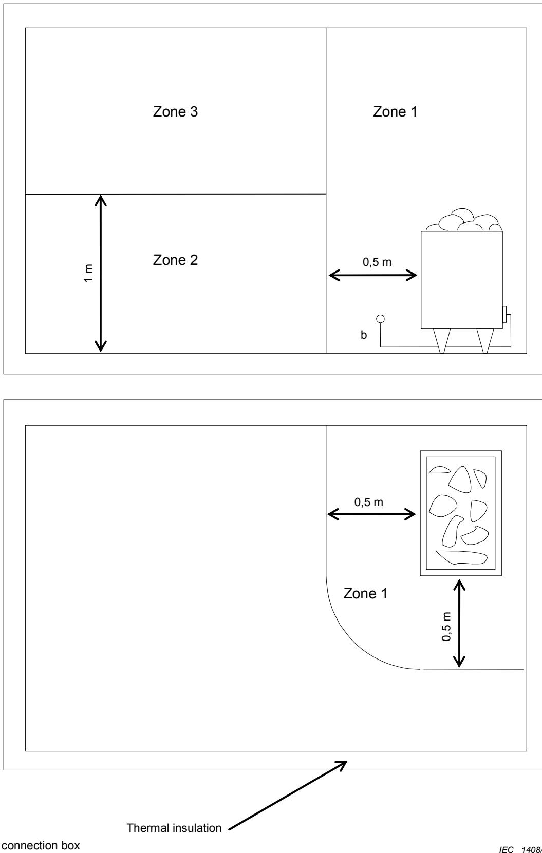
Figure 703 – Zones of ambient temperature
