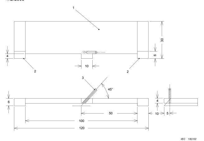
NOTE Jig body is made from insulating material.
