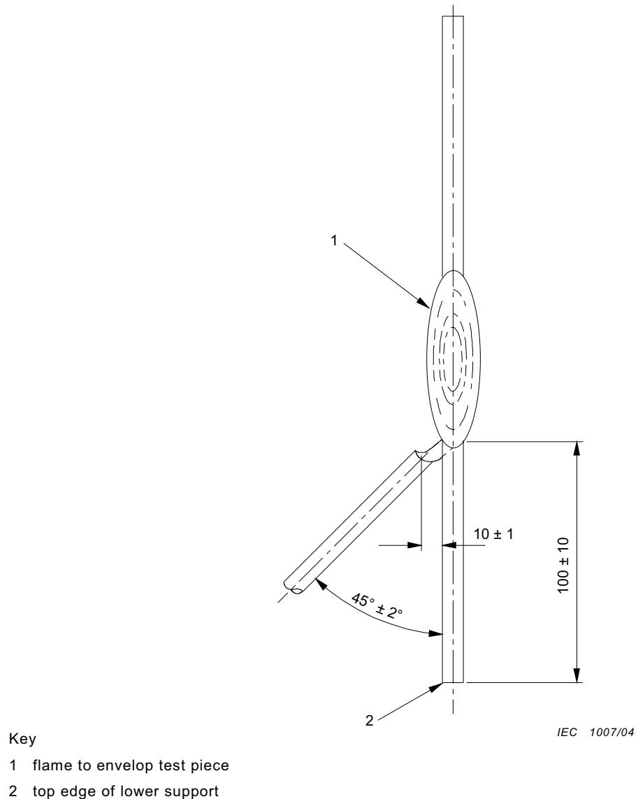
**Figure 4 – Application of burner to test piece (optical fibre cable)**
