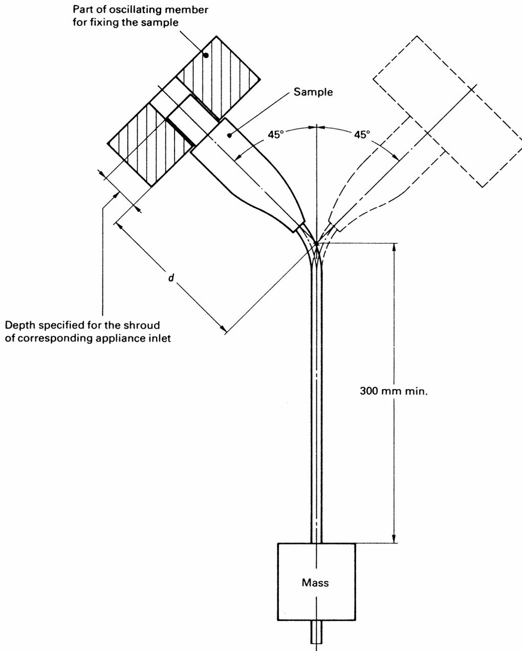
Figure 17 – Apparatus for the flexing test (see 22.4)
