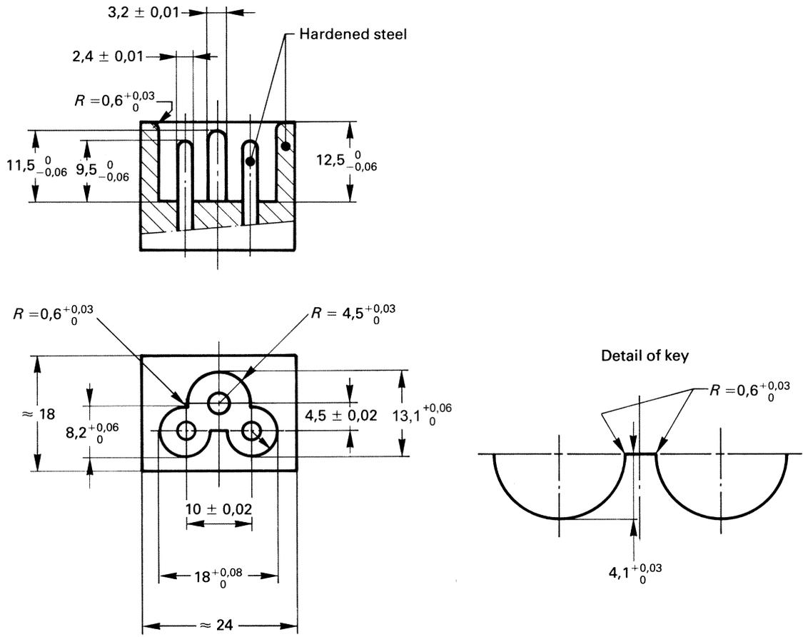
Figure 4 – "GO" gauge for connectors to standard sheet C5 (see 9.1)
