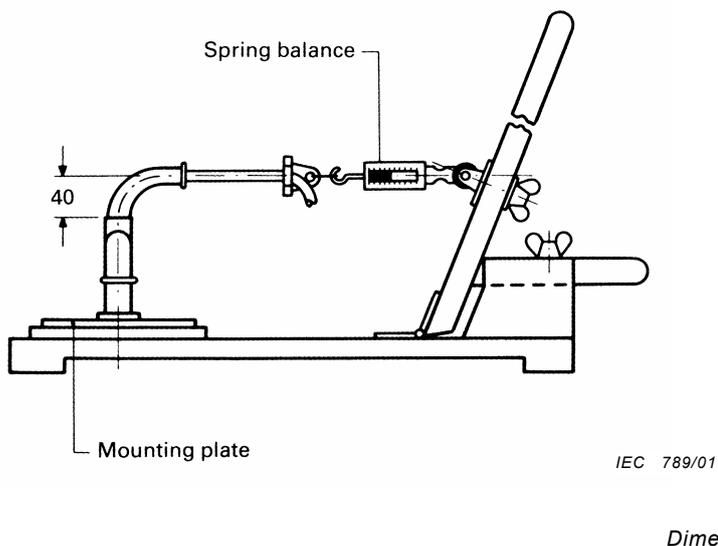
Figure 19 – Example of apparatus for pulling test (see 23.3)
