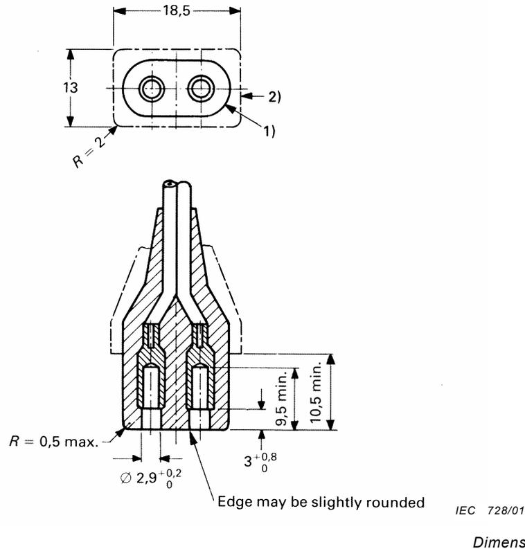
The centre distance and the design of the contacts as well as the dimensions and the design of the front part shall be such that
