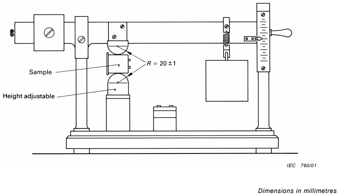
Figure 20 – Example of apparatus for pressure test on shrouds (see 23.4)
