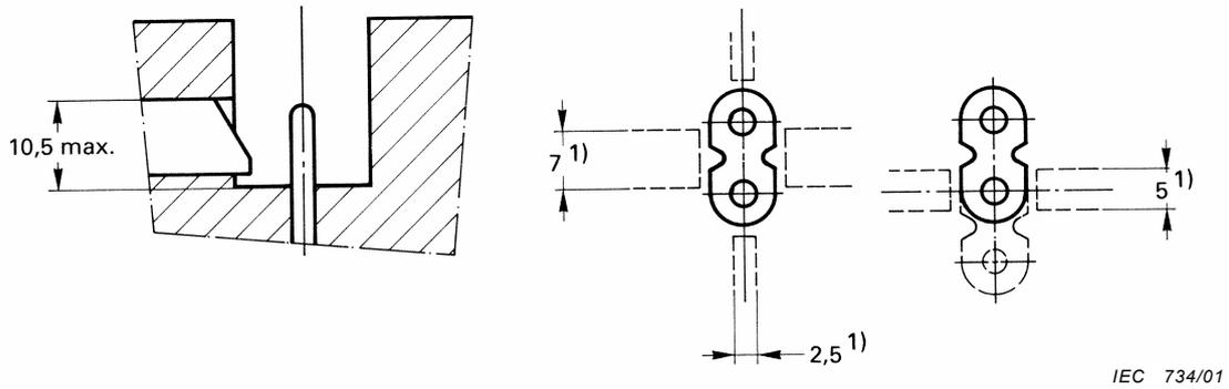
The operation of the switch shall be effected 1,5 mm before full engagement of the connector
