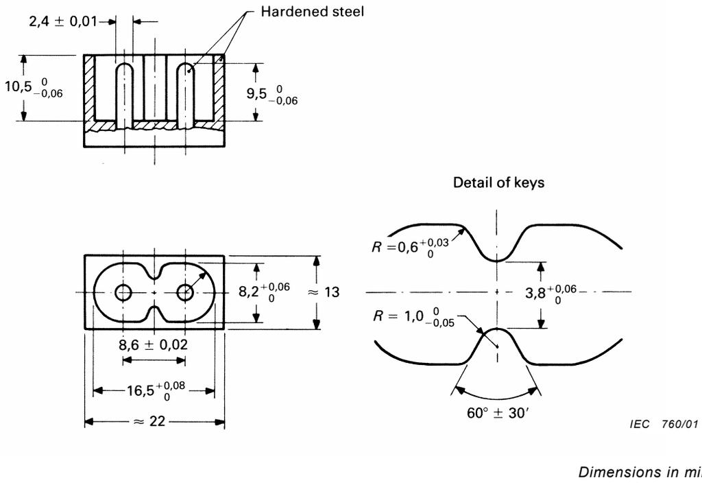
It shall be possible to insert the connector fully into the gauge with a force not exceeding 60 N.
