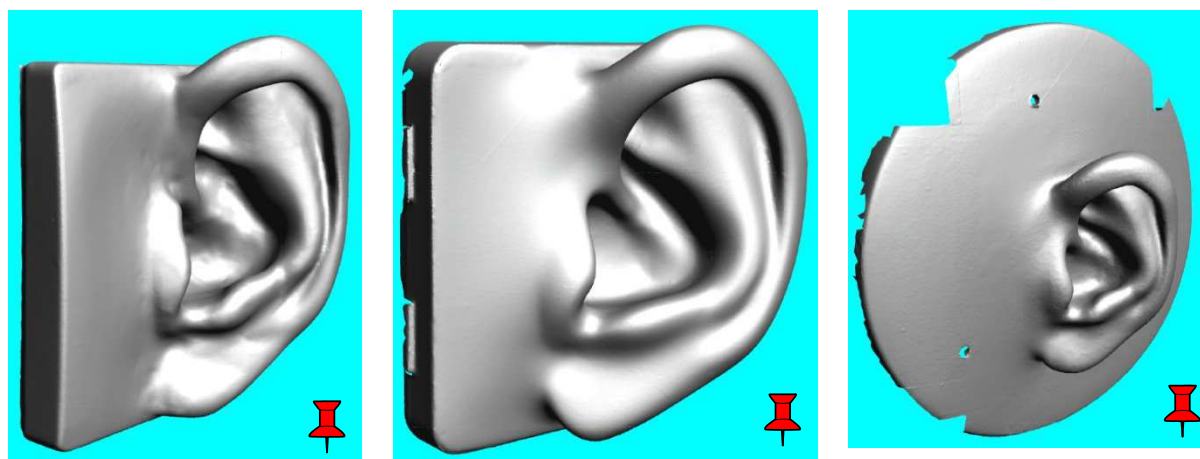
a) Pinna simulator for the anatomically shaped manikin example given in Annex A
