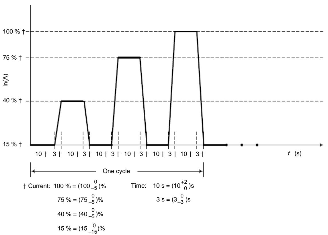
**Figure 101 – Current of test cycling**
