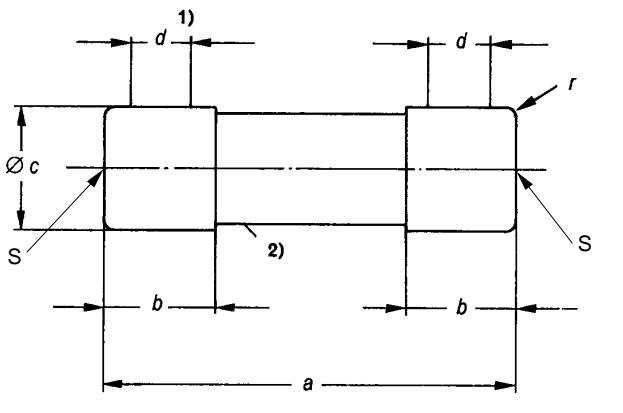
Measuring points S for power dissipation tests.
