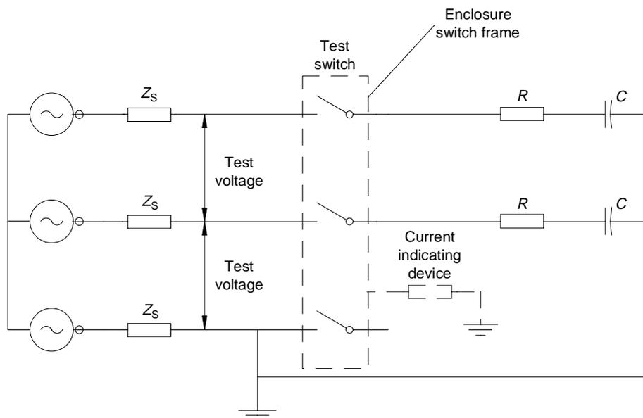
**Figure 9 – Three-phase test circuit for cable-charging breaking current tests under earth fault conditions, for test duty 6b**
