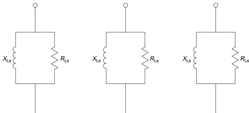
Figure 1c - Star load connection
