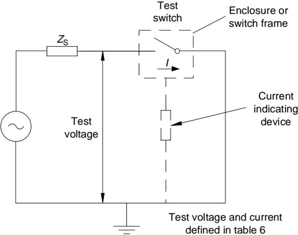
**Figure 6 – Single-phase test circuit for short-circuit making current test for test duty 5**
