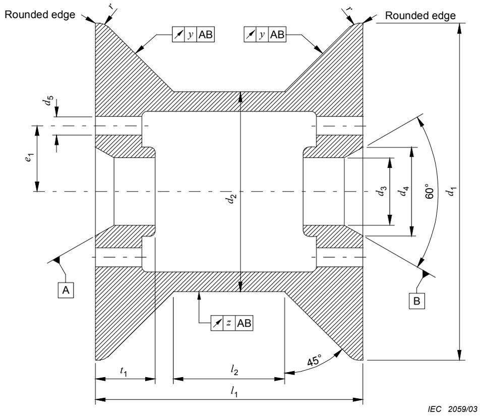
Figure 1 – Cylindrical barrelled delivery spool with conical flanges
