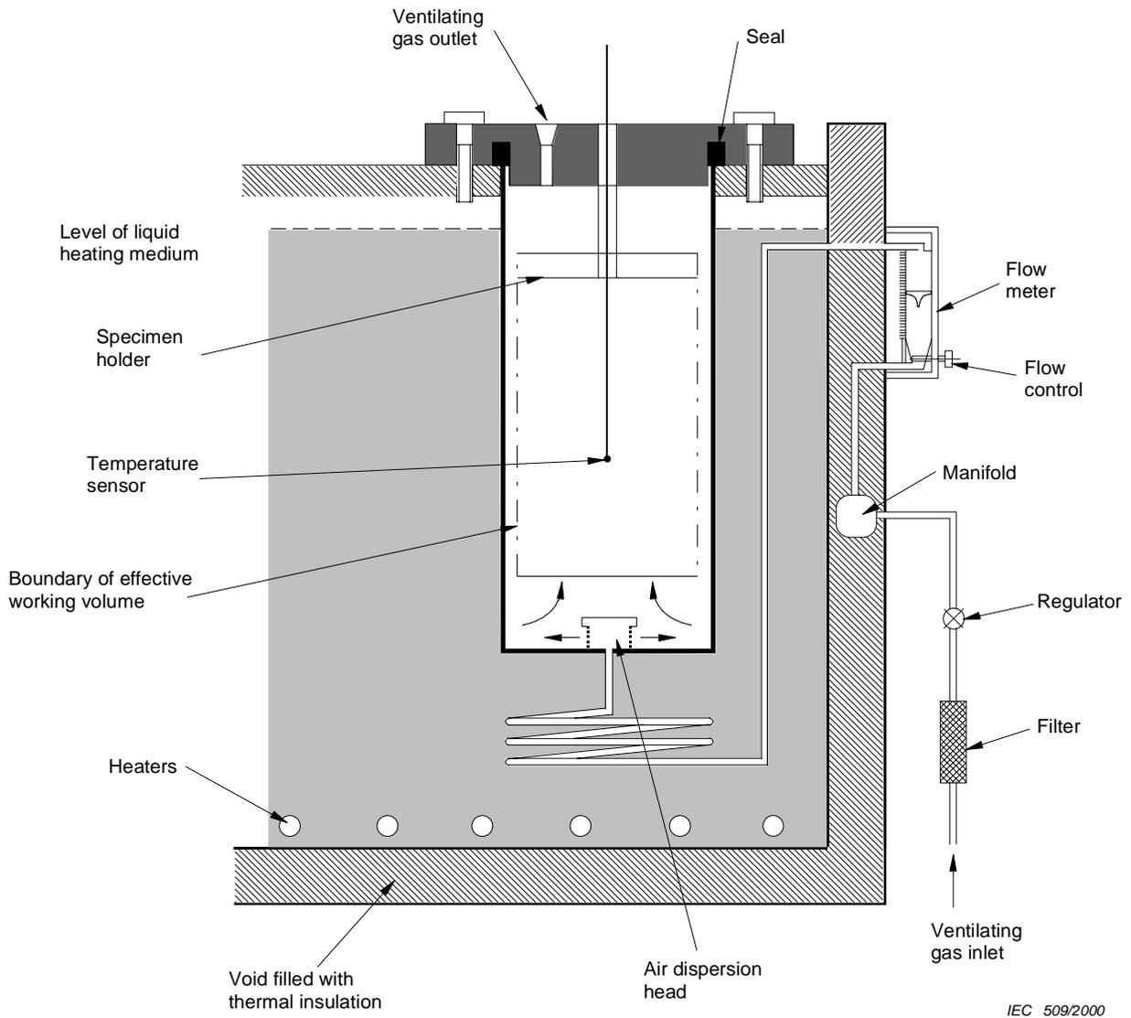
Figure 1 – Cell of a multi-chamber oven using a liquid heating medium
