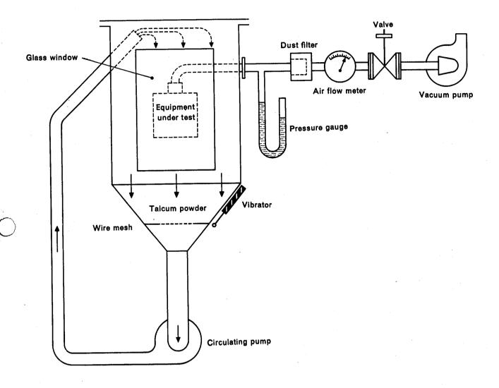
Fig. 2. — Equipment to prove protection against dust.
