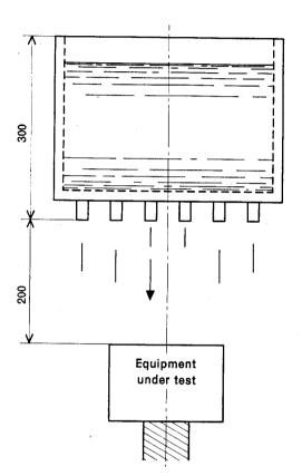
Layers of sand and gravel to regulate flow of water, these layers being separated by metallic gauze and blotting paper.
