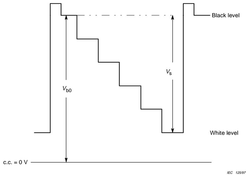
Figure 38 – Measurement of black level stability
