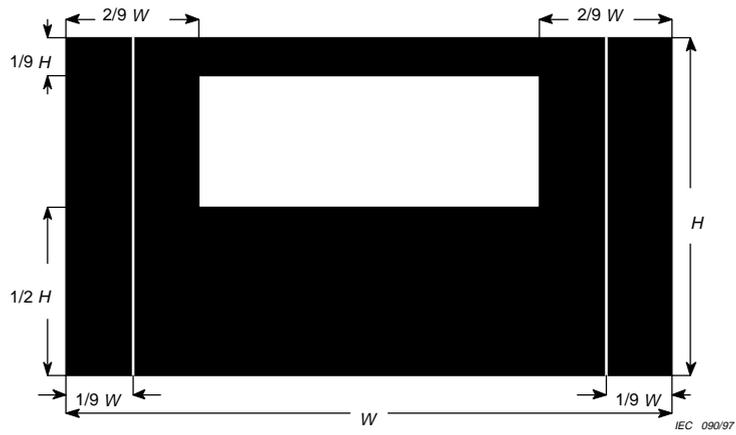
Figure 7a – Line and window pattern
