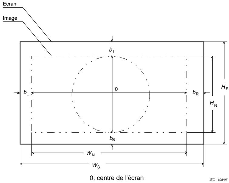
Figure 21 – Insuffisance de balayage
