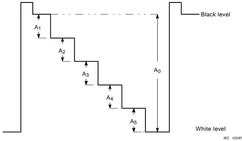
Figure 36 – Measurement of amplitude non-linearity
