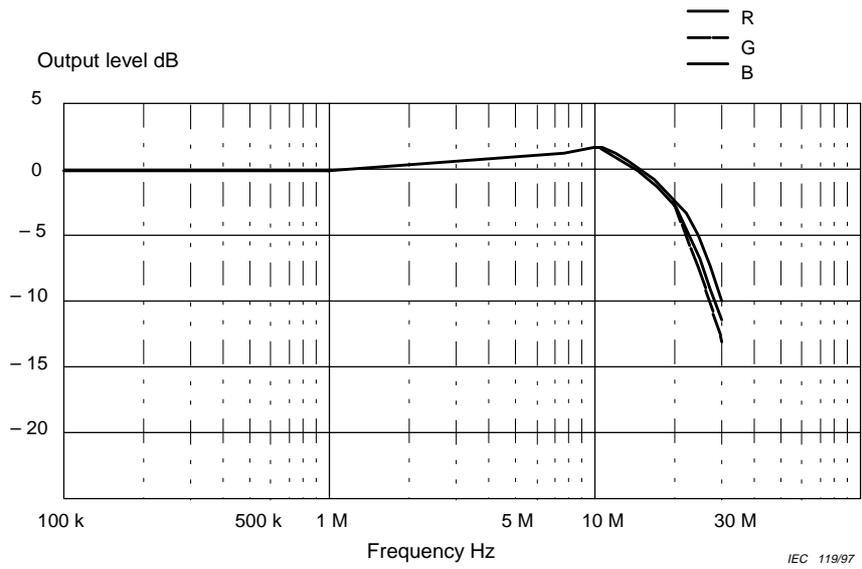
Figure 32 – Example of amplitude frequency characteristics
