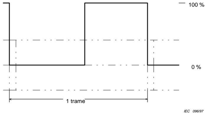
Figure 11b – Signal de barre horizontale
