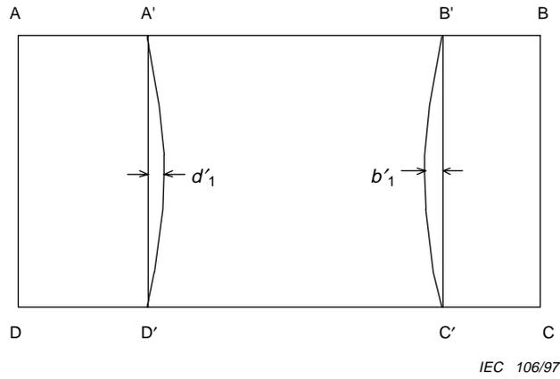
**Figure 19 – Inner distortion**
