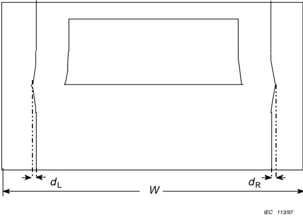
Figure 26 – Local picture distortion
