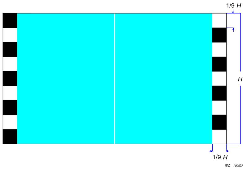
**Figure 14 – Checkered pattern signal**
