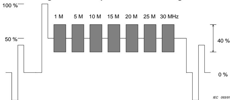
Figure 9 – Multiburst signal
