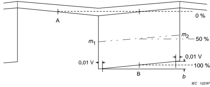
Figure 35 – Field rate square-wave response
