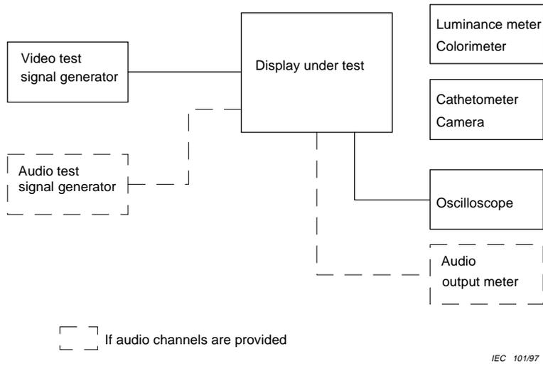
**Figure 15 – Notional block diagram of measurement setup**
