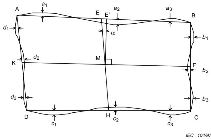
Figure 18a – Points for measuring outline distortion values
