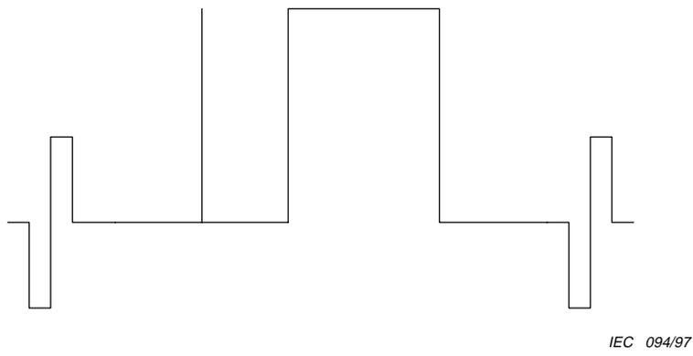
Figure 10 – 2T pulse and bar signal
