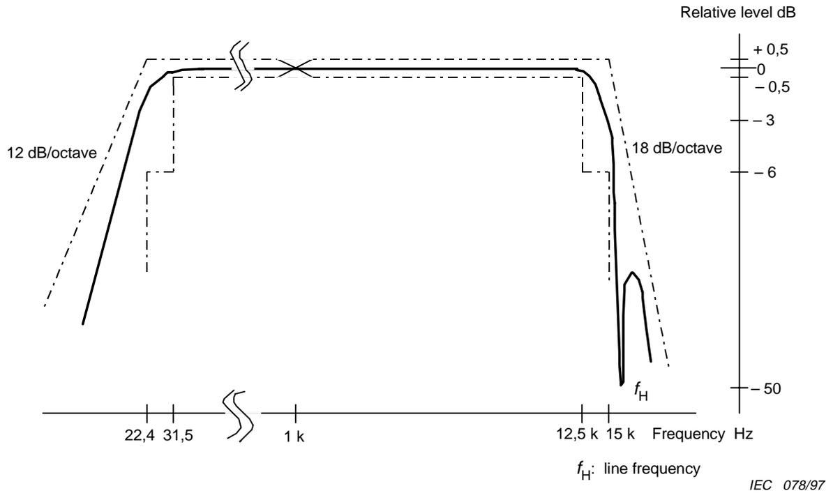
Figure 2 – 22,4 Hz to 15 kHz bandpass filter
