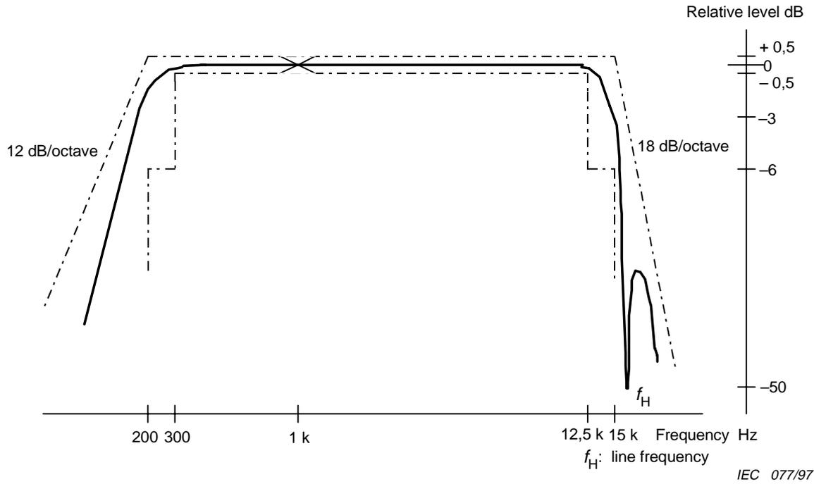
Figure 1 – 200 Hz to 15 kHz bandpass filter
