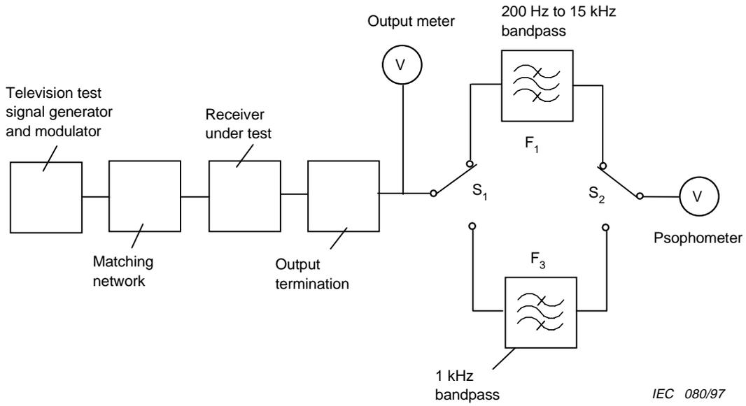
**Figure 4 – Measurement of signal-to-noise ratio**
