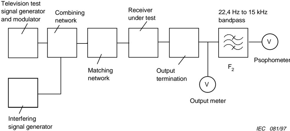
**Figure 5 – Measurement of wanted-to-unwanted r.f. signal ratio**
