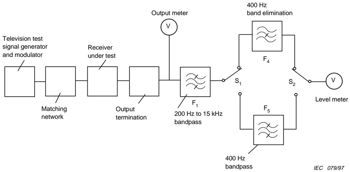
**Figure 3 – Measurement of amplitude modulation suppression ratio**
