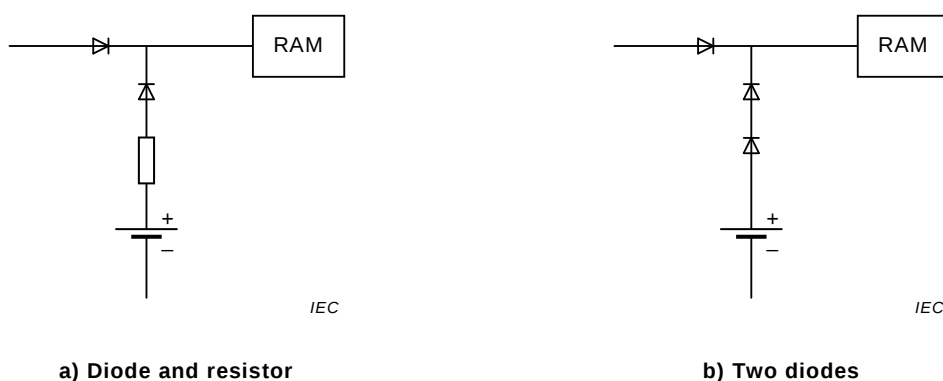
Figure 8 – Examples of safety wiring for charge protection
