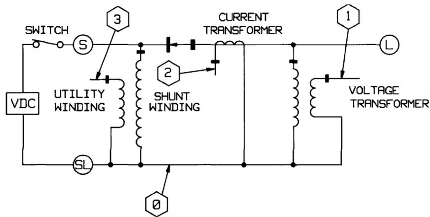
**Figure 8—Voltage regulator connected for polarity testing;
