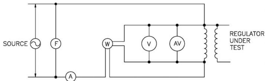
**Figure 12—Connection for no-load loss test of single-phase voltage regulator without instrument transformers**
