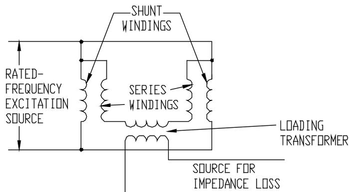
Figure 18—Example of loading back method: Single phase
