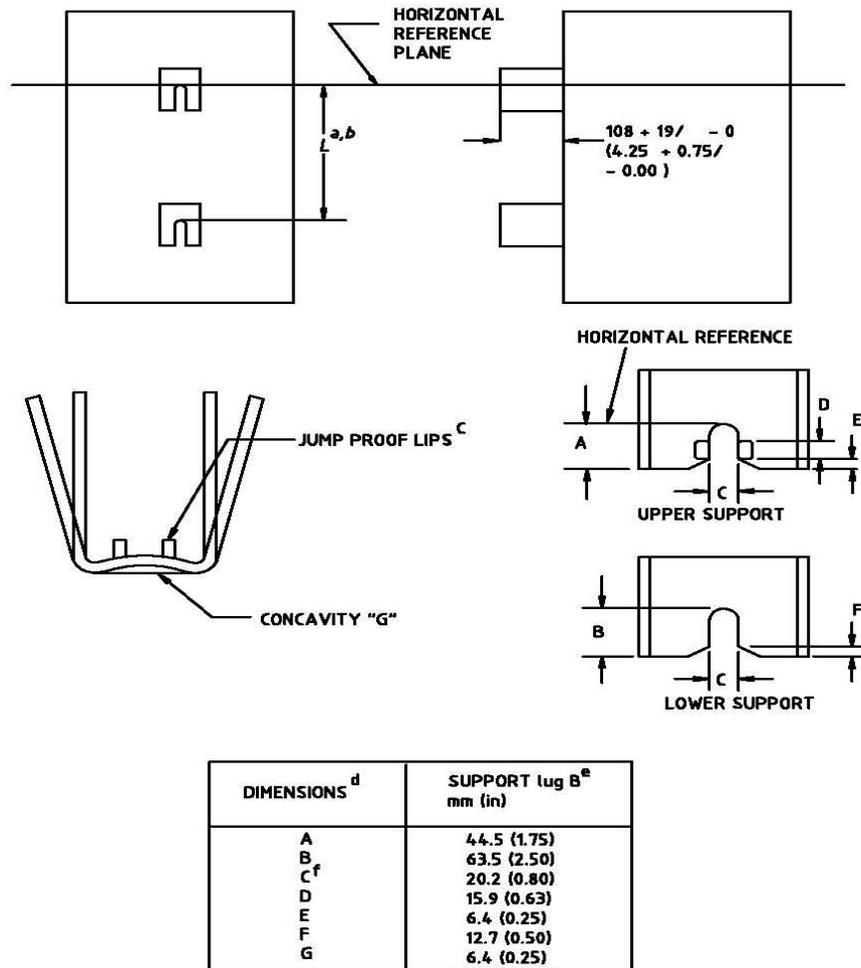
NOTE—Unless otherwise noted, all dimensions will have a tolerance of  $\pm 2$  mm (0.063 in). All dimensions are given in millimeters. Dimensions in parentheses are given in inches.
