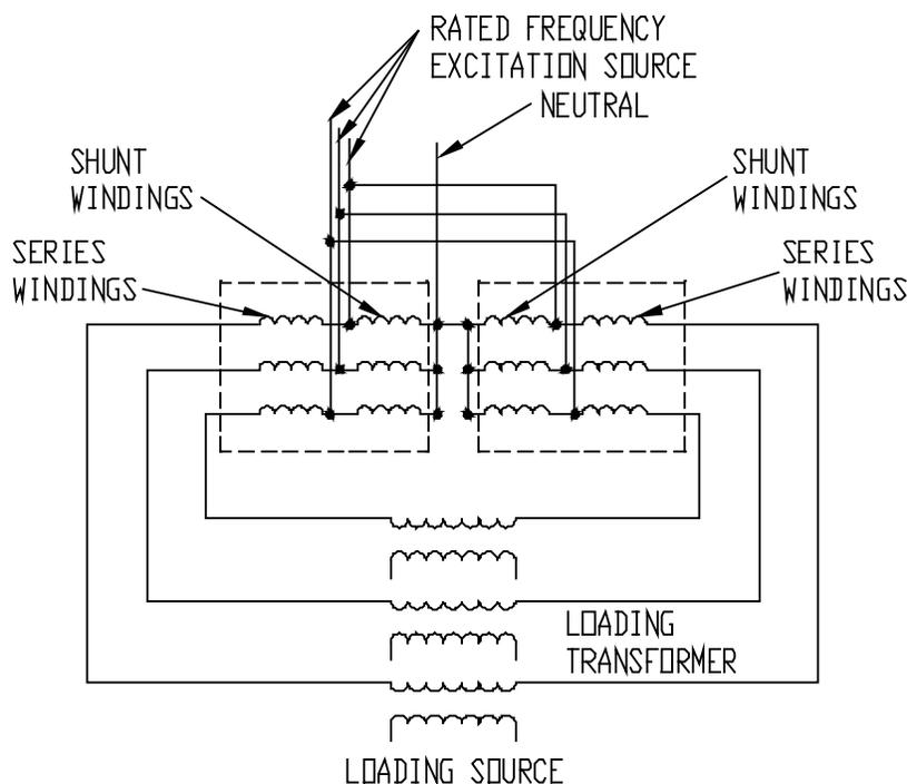
**Figure 19—Example of loading back method: three phase**
