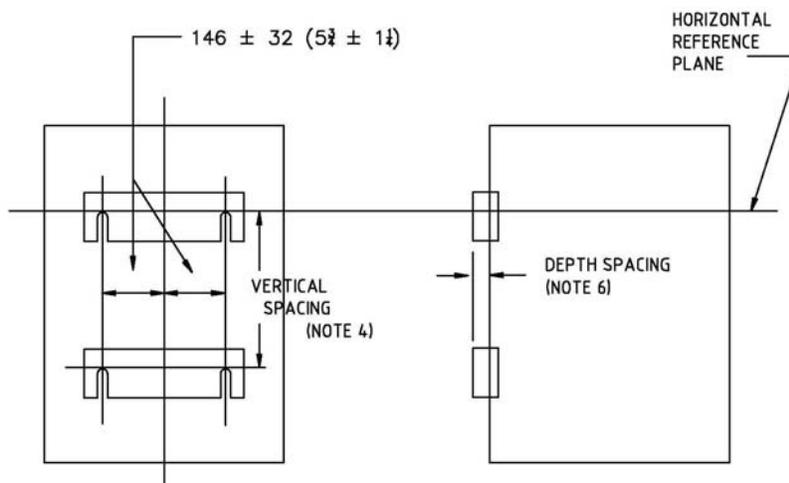
NOTE 1—Support lugs attached to voltage regulator with provisions for bolting on Type-C adapter plates for direct pole mounting.
