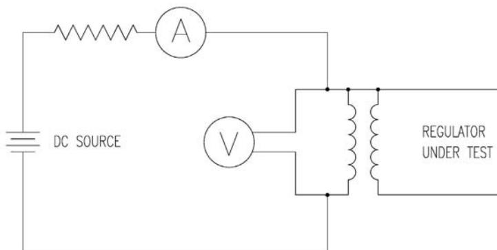
**Figure 7—Connections for voltmeter-ammeter method of resistance measurement**
