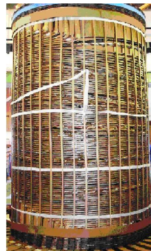
Figure B.18 – Frequency response of a tap winding before and after partial axial collapse and localised inter-turn short-circuit with a photograph of the damage
