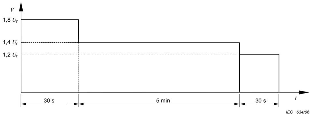
Acceptance levels: 50 pC at  $1,2 U_r$ ; 100 pC at  $1,4 U_r$  with  $U_r$  = rated voltage.
