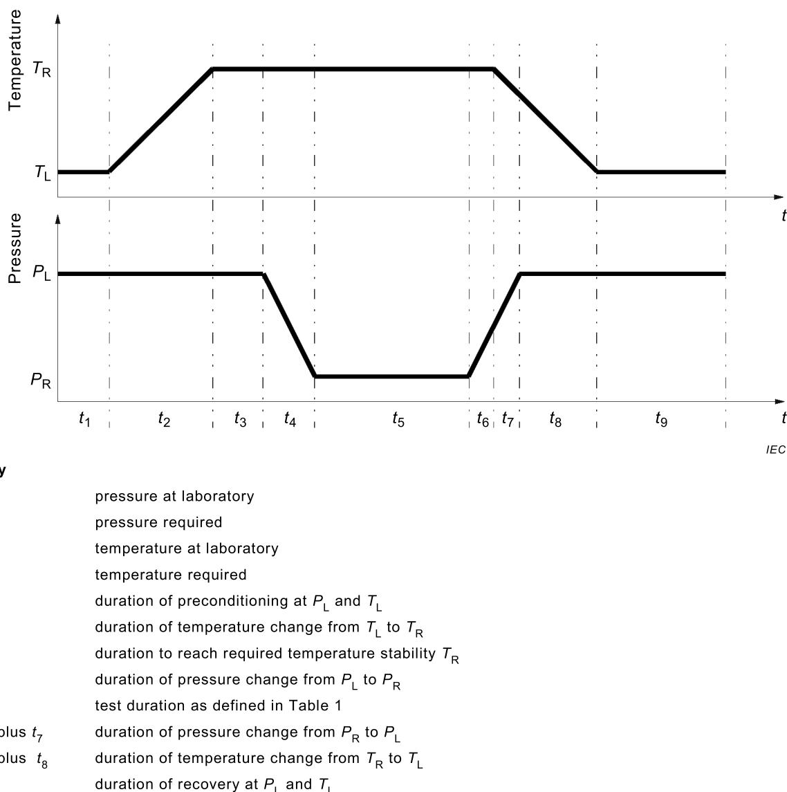
**Figure 2 – Example of test sequence with dry heat and low air pressure**
