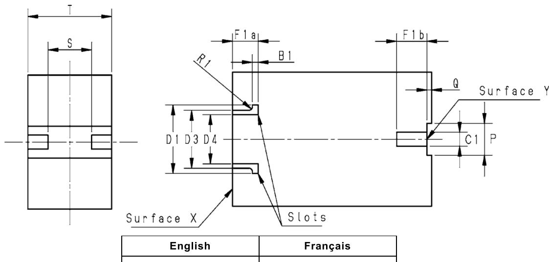
PURPOSE: To check pin dimensions of cap GX16t-5.
